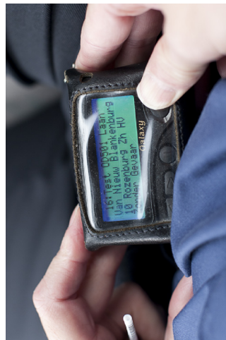
Figure 3.13. The same incident message in Figure 3.12 was also sent to the pager using P2000 one-way communications network.
