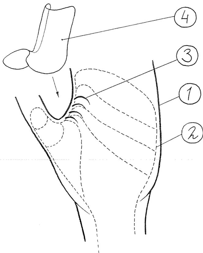
**Figure 2.** Heat-wire treatment setup. Electrical resistance wires are placed in the region where the glove is forced to stretch most. 1=glove, 2=internal mold, 3=heat wires, 4=external mold.
