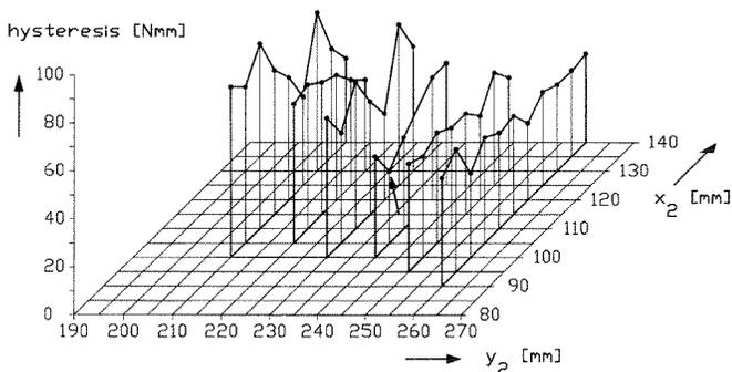
**Figure 10.** Graph of hysteresis as a function of cone motion driving axis orientation. The position of bearing  $\oplus 2$  is used as a measure for the thumb axis orientation. The minimum is located at  $(x_2, y_2) = (105, 240)$ , its value is 32 Nmm. This position corresponds to a movement with uniform glove stretching.
