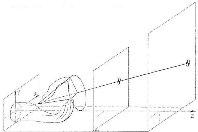
**Figure 5.** Schematic view of the experimental setup for the thumb movement optimization. The cone that is described by the thumb is clearly visible. The externally mounted driving axis is hinged by two bearings, marked with  $\oplus$ .
