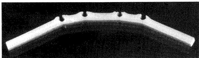
**Figure 3.** Section of the glove, perpendicular to the grooves. No material is removed, but the glove section is reshaped.
