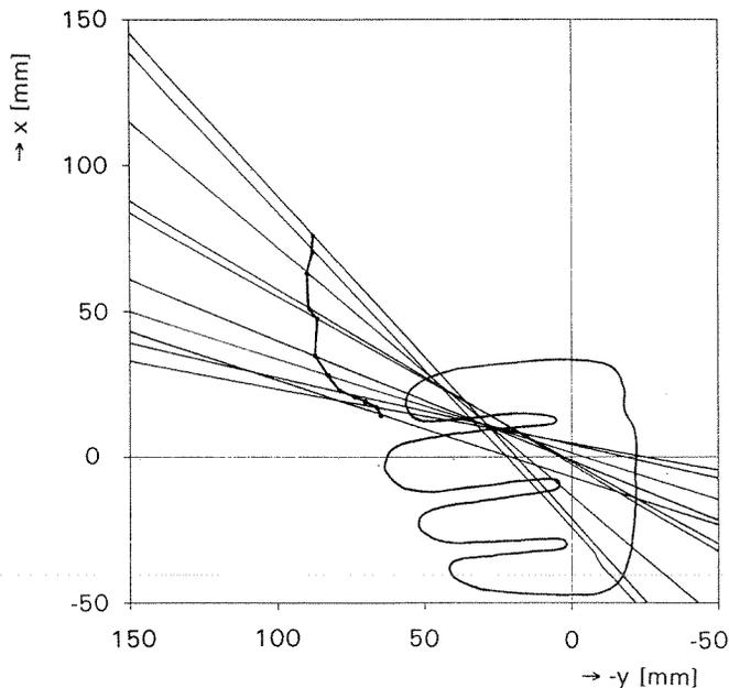
**Figure 9.** Proximal view of test prosthesis with bent fingers, showing the cosmetic thumb movement that can be approximated by a cone motion. The trajectory of the tip of the thumb and center lines of the corresponding thumb positions are shown.
