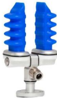
Figure 2-4: Mgripper by Soft Robotics inc. [48,42].
