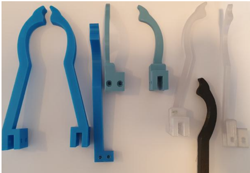
Figure 5-1: Overview of rigid pinch gripper prototypes.
