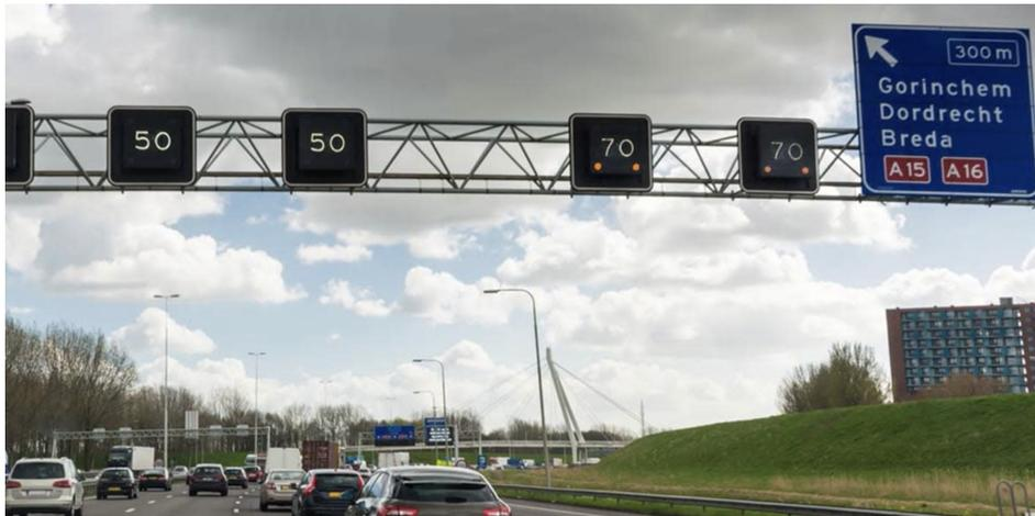
**Figure 2-3:** VSLs used on a A15/A16 highway in the Netherlands [3].
