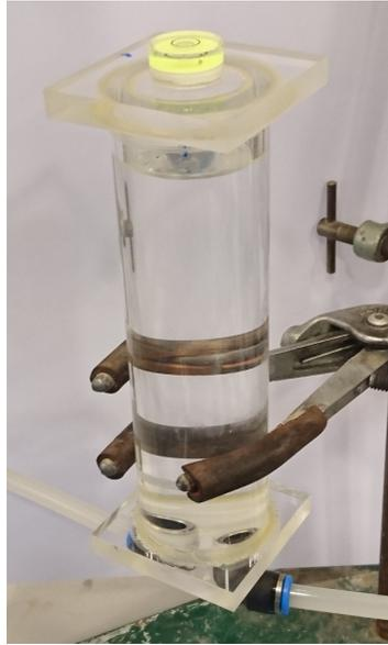
Figure 3.8: Gas trap connected to the back-pressure line of Rowe cell
