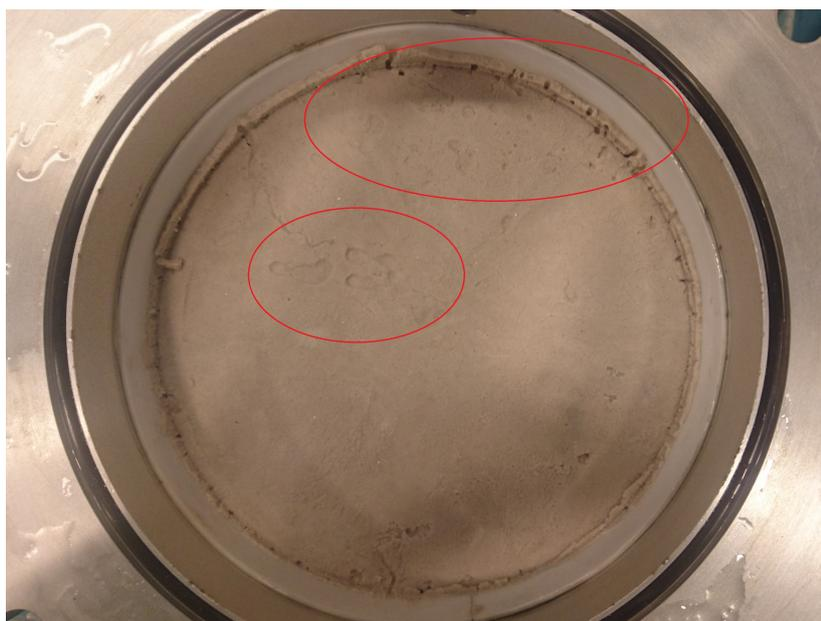
Figure 4.9: Visible gas pockets on surface of a treated Geba-M6 84-16 sample and bulging of the soil around the edge of the cell - after disassembly
