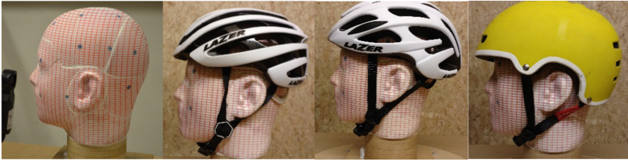
Fig. 4. (i) Thermal manikin or nude headform (ii) open helmet with internal channel (OHIC) (iii) open helmet without internal channels (OHWIC) (iv) closed helmet (CH)
