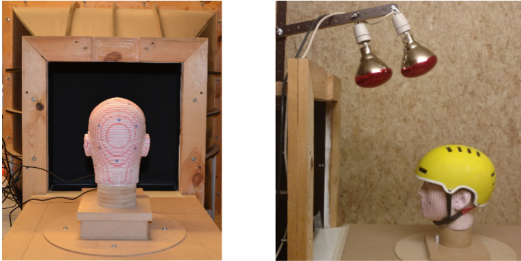
Fig. 3. (i) Thermal manikin positioned at the outlet of the wind tunnel (ii) radiative heat transfer setup with heat lamps
