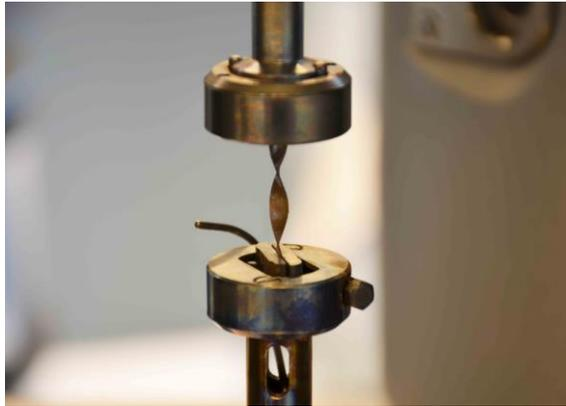
**Figure 5.6.** The torsion mode test setup in a Thermofisher Haake MARS III rheometer equipped with a solid clamp geometry.
