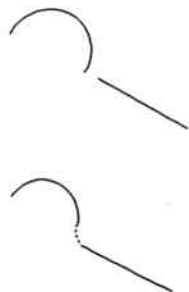
Figure 23 without spacing, difficult matching of two sections (upper), with some space, smooth matching possible (lower).
