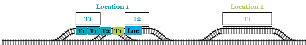
Railway State 2.20: The train arrives at Terminal 1 of the first destination. The last cars will be placed such that they can be decoupled and the train can continue in one go.
