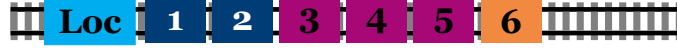
Railway State 4.2: Example train with six cars for three different destination groups.
