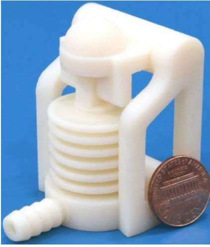
Fig. 3: MacCurdys' 3D-printed bellow produced as a single part with pre-filled with printable liquid internal channels [15].
