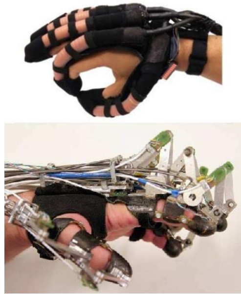
Fig. 2: Top: Soft actuated hand exoskeleton by Polygerinos et al. [24], bottom: hand rehabilitation exoskeleton device by Wege et al. [26].
