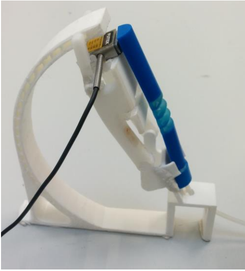
Fig. 17: Testing configuration. Pressurized air is fed to the actuator, while the force sensor measures the force that the actuator is generating at the tip. The main base have a rotational locking system every 5 degrees (arc) allowing to also test a second feature: the ROM, with accuracy of 5°.
