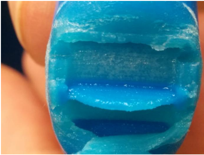
Fig. 24: Corrosion of the inner walls of the actuator's chamber, due to chemical cleaning procedure of the support material. The corrosion has weakened the soft material to a point that it failed without pressurizing it.
