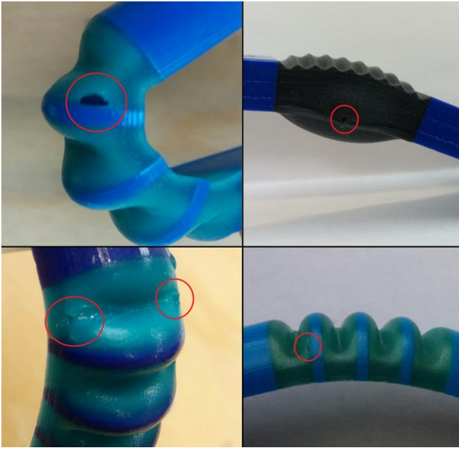
Fig. 23: Failure points of 4 different actuators (after testing). Even though four are presented, in all cases the failure point was located either on the side or in-between two chambers (on the top of the actuator).
