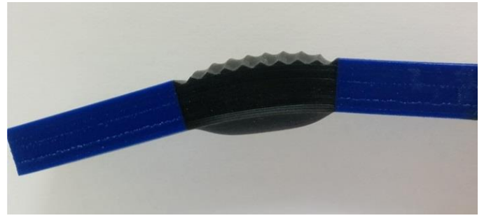
Fig. 13: First prototype of a 3D-printed soft actuator with soft area (black material) adjusted to be 70% stiff while the hard area (blue material) to be 100% stiff. The actuator is under 1.2 bar of air pressure.
