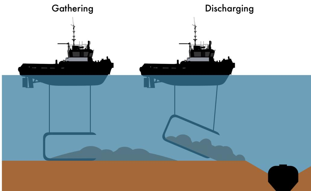
Figure 27: Visualization of improved shark teeth trailer working principle
