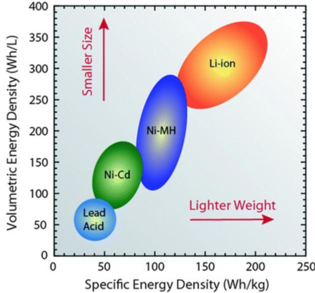
Figure 24: Energy density of different batteries. Source: (Epectec, 2020)
