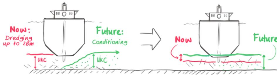
Figure 10: The effective depth. Source: PRISMA
