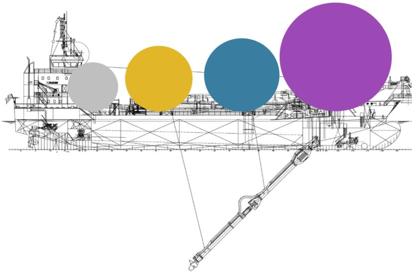
Figure 4: Visualization of required volume per fuel. Grey: diesel, yellow: methanol, blue: hydrogen, purple: lithium-ion batteries
