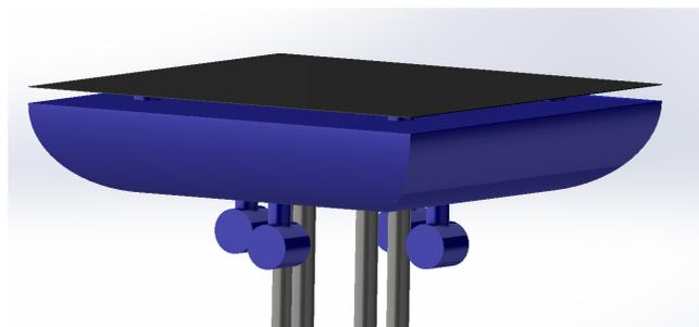
Figure 14: Poolbuoy Carrier Vessel with PV-cell on top
