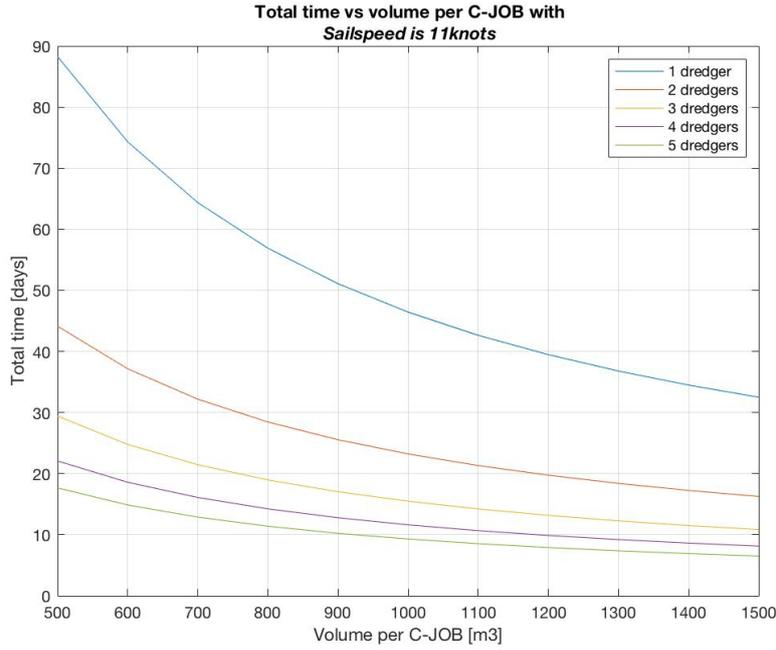
Figure 23: Plot to determine initial parameters of autonomous submerged dredger.
