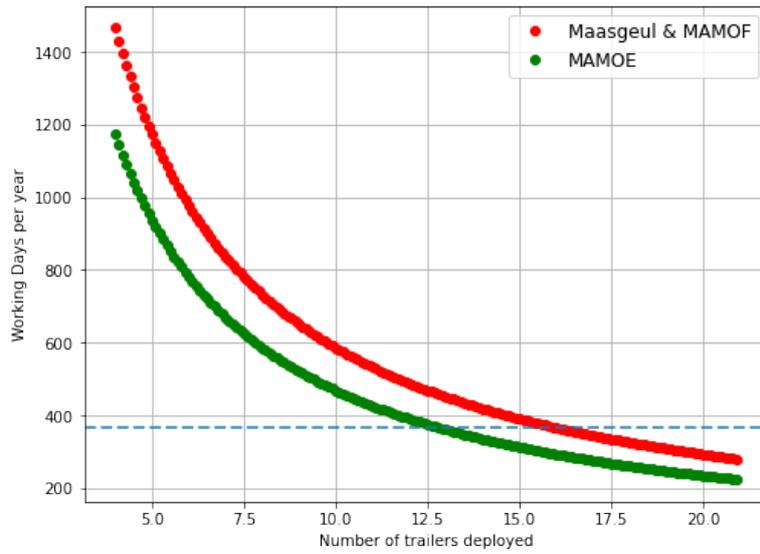
Figure 18: Working days per year vs. Number of trailers deployed
