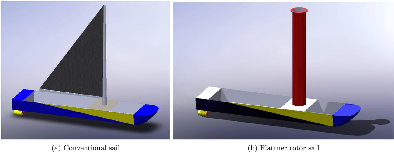
Figure 6: Design visualization for sailing autonomous barges.
