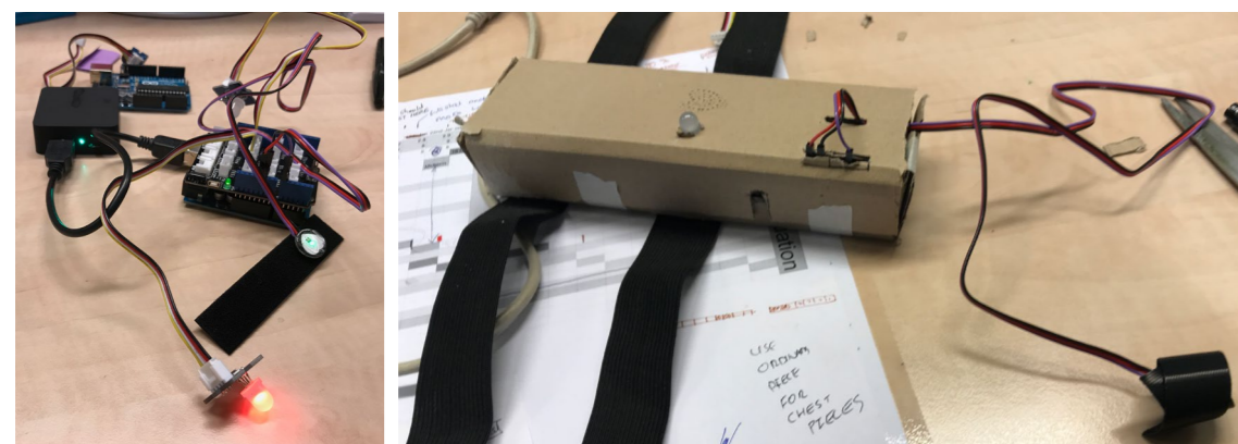
Figure 3.26: Heart rate Prototype: (top) Components integrated in cardboard form, (bottom left) loose components (bottom right) Completed prototype.
