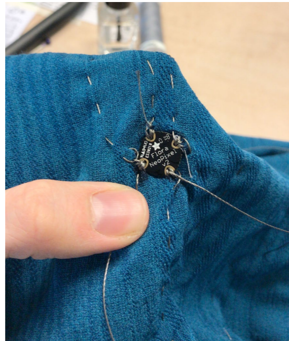
Figure 4.11: Sealing neopixels with nail varnish
