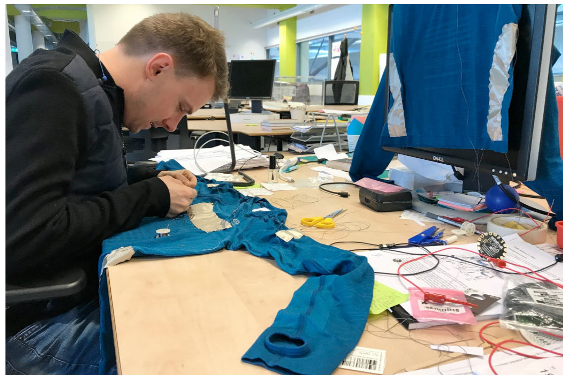
Figure 4.12 Sewing touchpads onto garment
