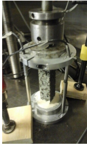
Figure 6. Adjusted sample with loading plates, transducers and clampers
