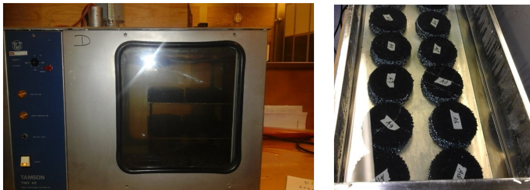
Figure 7. Bath conditioning of the samples for different time intervals
