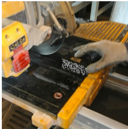
Figure 13. Sawing of the beams from the cylinder sample.
