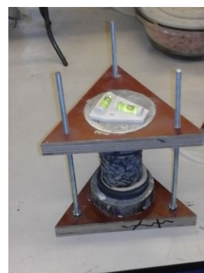
Figure 17. The apparatus used for alignment and the 3-D rings
