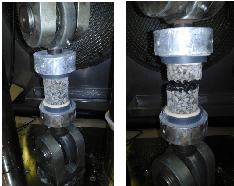
Figure 18. Sample before and after the interlayer bonding test
