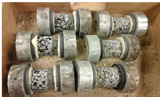
Figure 16. The glued specimens stored on sand-layer in a climate chamber
