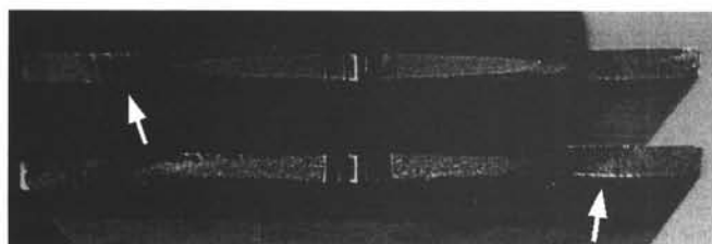
Fig. 6: Fracture surfaces of specimens of 2024 (top) and 7075 (bottom), tested with load spectrum 1.
