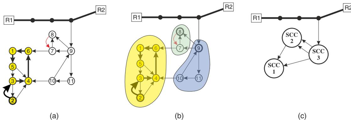
**Fig. 3.** Digraph transformation to DAG: (a) start the DFS; (b) detected SCCs; and (c) newly formed DAG.
