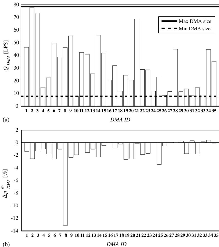
**Fig. 10.** Results for each DMA in preferred solution, Sol-9: (a) average DMA consumption; and (b) relative change of mean average pressure.
