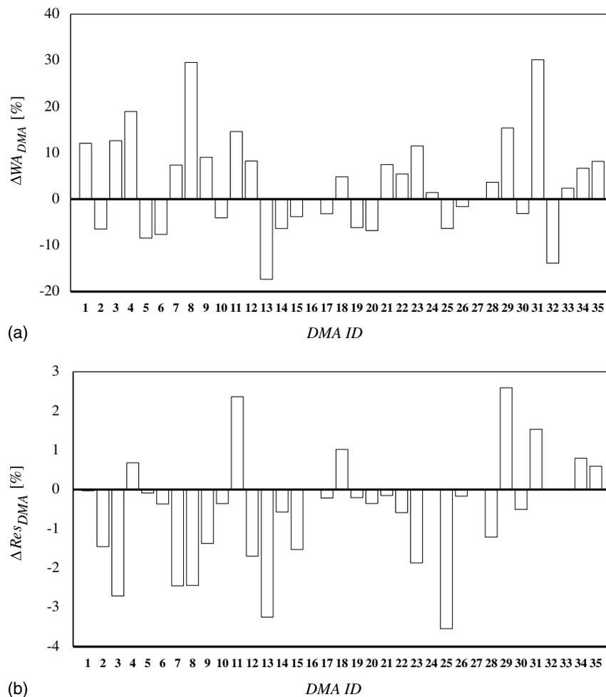
**Fig. 11.** Results for each DMA in selected preferred solution, Sol-9: (a) relative change of water age; and (b) relative change of resilience index.
