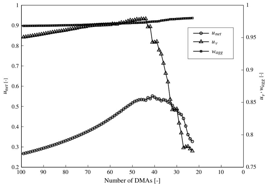
**Fig. 8.** Evolution of all three components ( $u_{net}$ ,  $u_v$ , and  $w_{agg}$ ) constituted in the network uniformity index ( $U$ ) in the last 77 aggregation steps.
