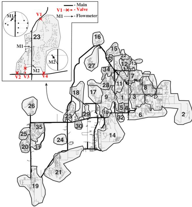
**Fig. 9.** Preferred sectorization solution, Sol-9, with 35 DMAs and detail of DMA 23.
