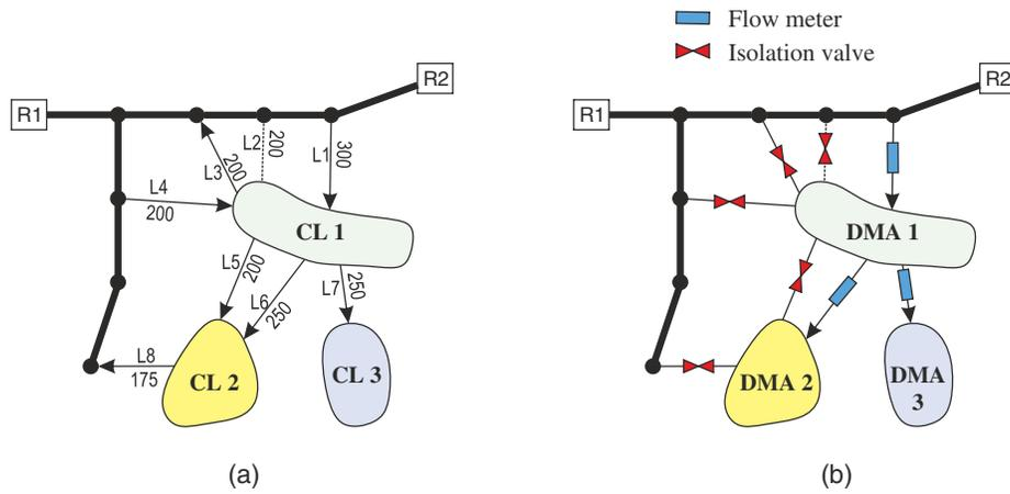
Fig. 6. Heuristics-based placement of flow meters and isolation valves (Stage 3-Step 1).
