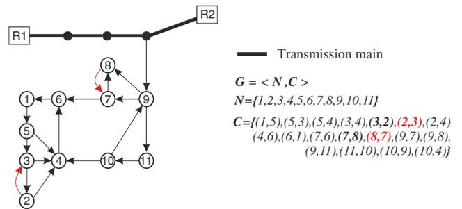
Fig. 2. Digraph presentation of a simple network with two sources and two undirected links.
