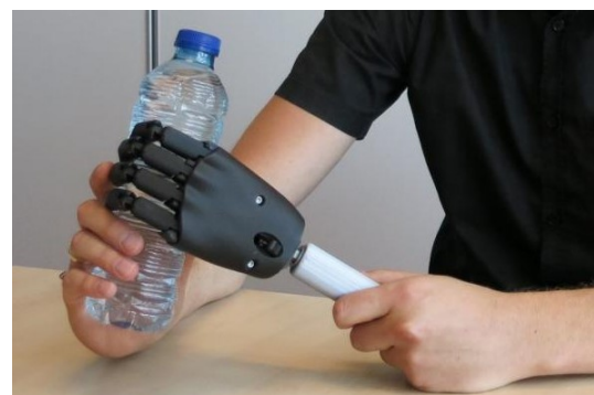
(b) The SGH without cosmetic glove, where the button on the back of the hand is visible, used to open the SGH [36].
