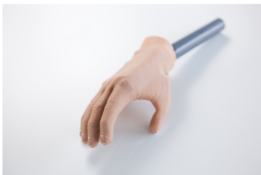
(a) The Self Grasping Hand (SGH) with cosmetic glove [1]
