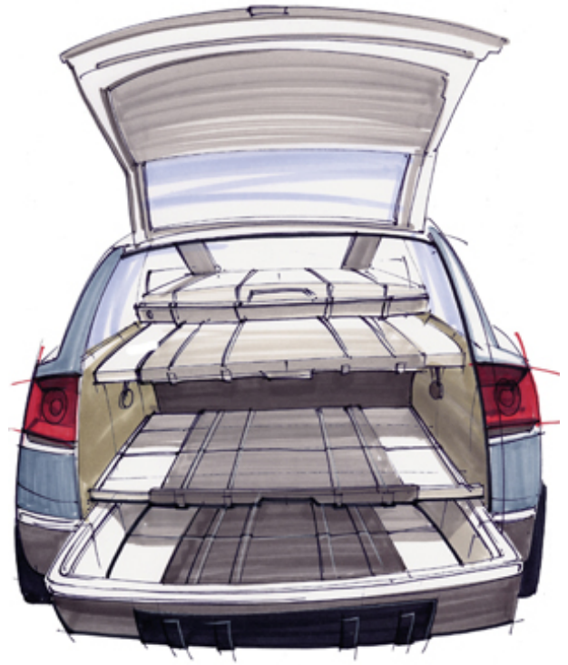
The design comprises four layers: clean at the top, dirty at the bottom.
