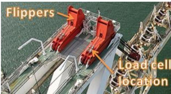
Figure 1.4 Flippers supporting the dead ends of hang-off cable with load cells. © Hans@Fotovlieger.nl.
