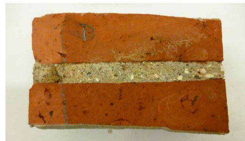
FIG. 4.21 Measurement of the impregnation depth / Photo: B. Lubelli
