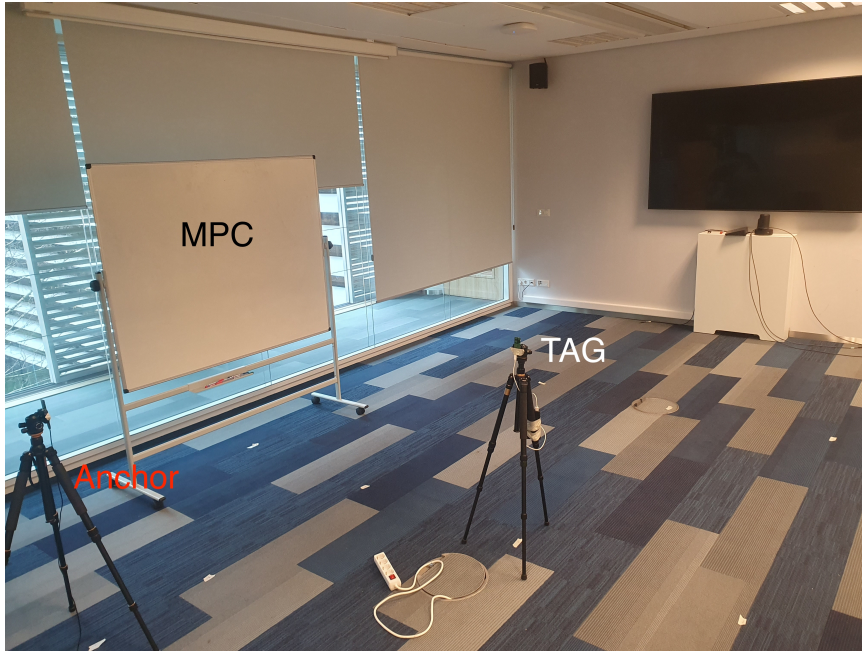
Figure 5.3: Indoor experimental setting of the anchor and the tag.
