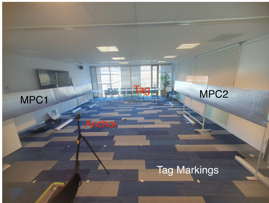
Figure 5.7: Experimental setting of anchor and tag with two MPCs.
