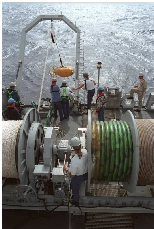
Figure 1.8: The CAPTAS array and the SOCRATES source being deployed from the aft deck of HNLMS Mercuur. (Photo P.A. van Walree)
