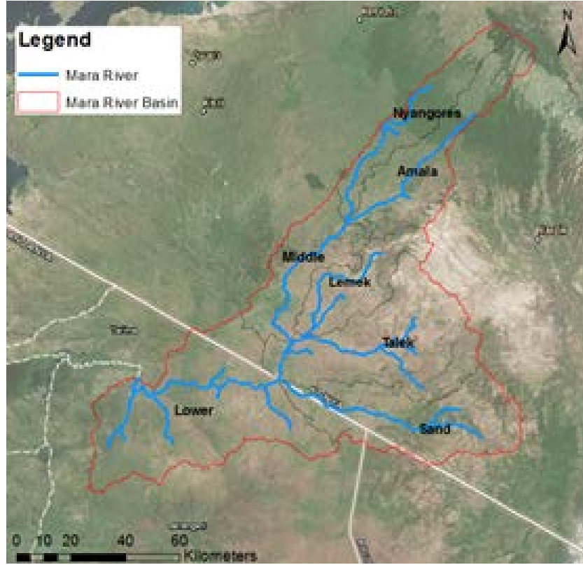
Figure A.5: Subcatchments defined in the hydrological model of Hulsman, 2015.
