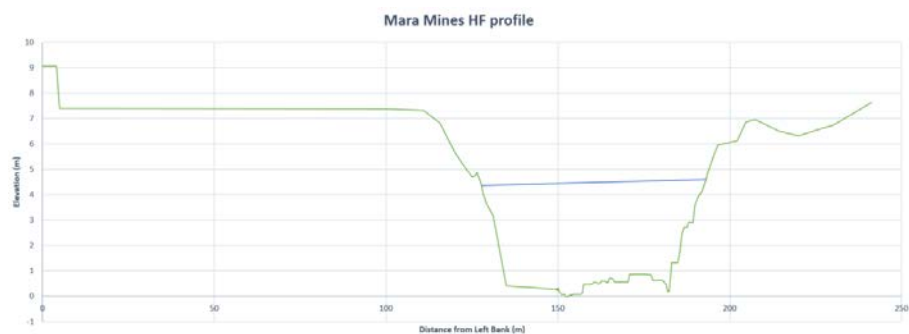
Figure C.4: Cross section Mara Mines measured during high flow with the Total Station
