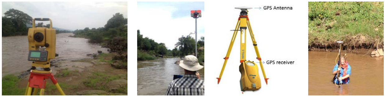
Figure 4.4: Cross section measurement equipment. From left to right: Total station of TopCon at Mara Kichwa Tempo, Measurement of cross section with the total station at Amala Kapkimolwa, Base station of Trimble R7 set-up and DGPS Rover used to measure the wet cross section at the Amala Kapkimolwa during low flow.
