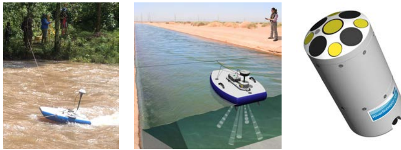
Figure 4.3: RiverSurveyor as used in the field (left), as prescribed in the manual of SonTek (Sontek2010) (middle) and the RiverSurveyor M9 ADCP sonde which sends out the sonar signals (right)
