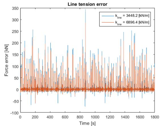
Figure 5-32 Line tension error, case 3: different line stiffness
