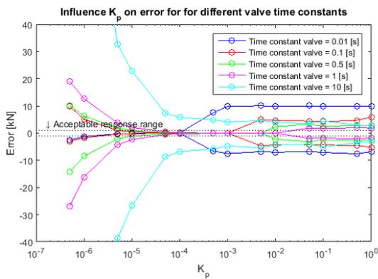
Figure E- 3 Hydraulic system, influence proportional gain,  $F_{amplitude} = 500$  [kN],  $F_{min} = -10$  [kN]
