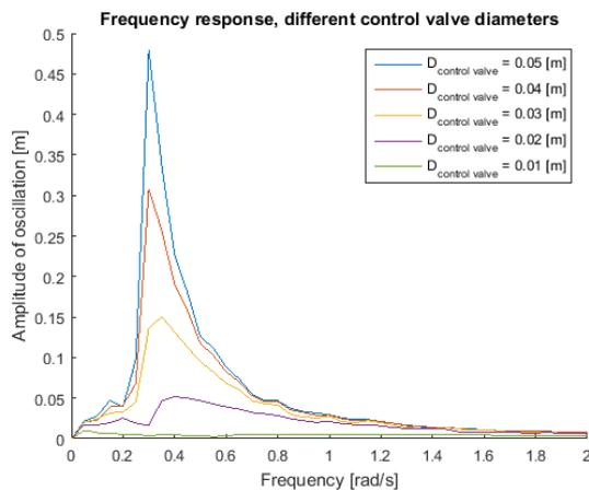
Figure 4-15 Frequency response, different control valve diameters
