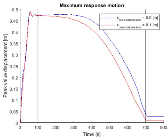
Figure 4-21 Maximum response motion, pre-compression fender
