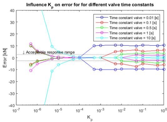
Figure E- 9 Hydraulic system, influence proportional gain,  $F_{amplitude} = 1000$  [kN],  $F_{min} = -500$  [kN]
