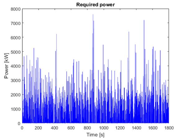
Figure 5-24 Required power, case 1: hydraulic actuator 1
