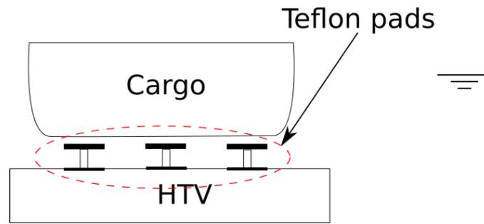
Figure 3-3 Teflon pads, schematic cross section
