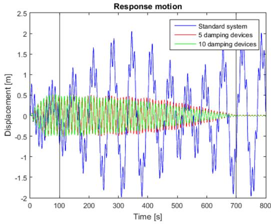
Figure D- 19 Response motion, irregular force case 2
