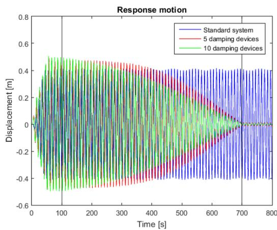
Figure D- 9 Response motion, different amount of damping devices
