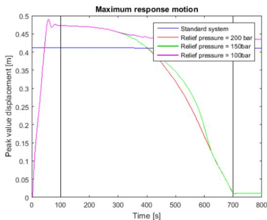
Figure 4-31 Maximum response motion, different relief pressures
