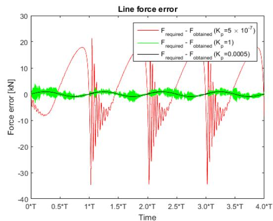
Figure 5-11 Hydraulic system, line force error
