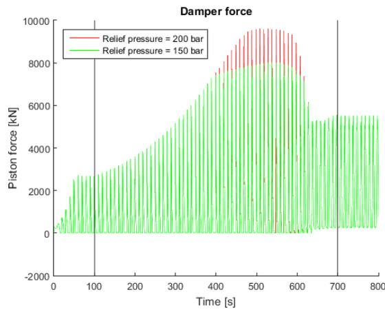
Figure 4-35 Damper force, different relief pressures (200 bar, 150 bar)
