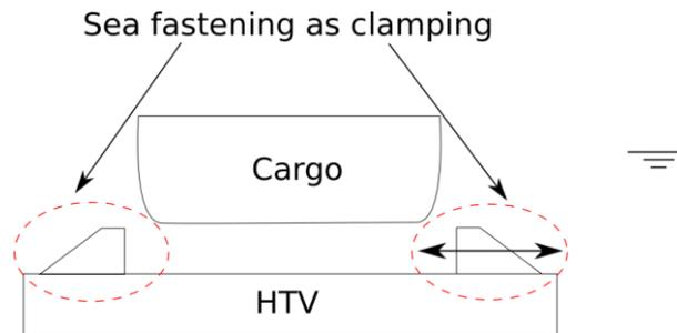
Figure C- 16 Third configuration, schematic cross section
