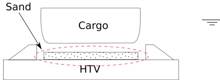
Figure C- 21 Sand as support system, schematic cross section
