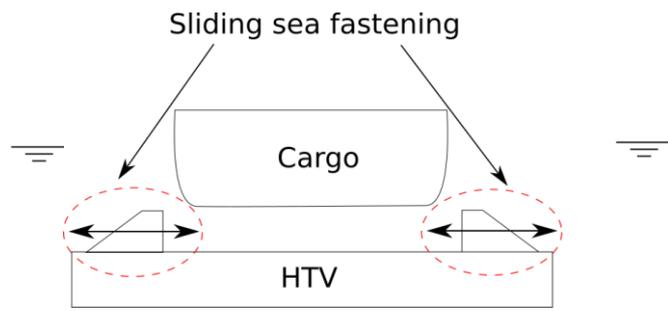
Figure C- 15 Second configuration, schematic cross section
