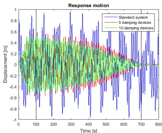
Figure D- 26 Response motion, irregular force case 3
