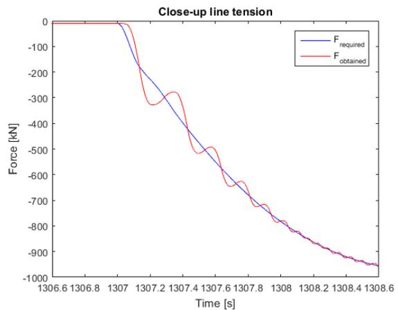
Figure 5-22 Close-up line tension around  $t = 1307$  [s], case 1: hydraulic actuator 1
