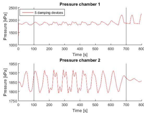
Figure 4-43 Pressure inside the cylinder chambers, excitation frequency close to the natural frequency of the standard system
