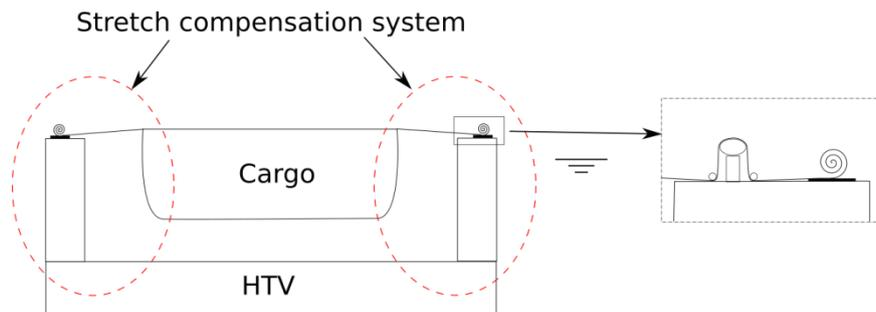
Figure 3-2 Stretch compensation system, schematic cross section
