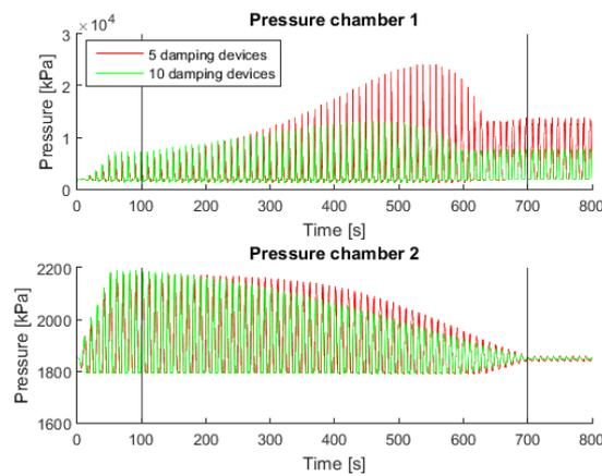
Figure 4-30 Pressure inside the cylinder chambers, different amount of damping devices
