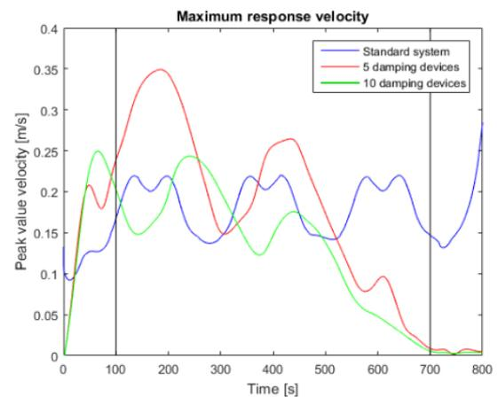
Figure 4-50 Maximum response velocity, irregular force case 1
