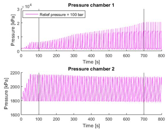
Figure 4-38 Pressure inside the cylinder chambers, different relief pressures (100 bar)
