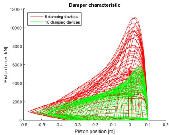
Figure D- 30 Damper characteristic, irregular force case 3
