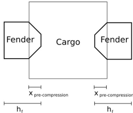
Figure 4-20 Schematic overview of pre-compression of the fender
