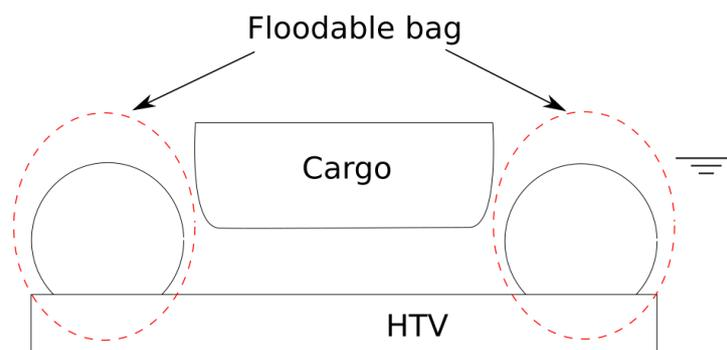
Figure C- 18 Floodable bag, schematic cross section
