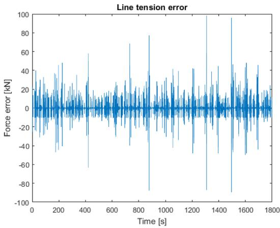
Figure 5-19 Line tension error, case 1: hydraulic actuator 1
