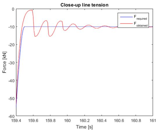
Figure 5-21 Close-up line tension around  $t = 159$  [s], case 1: hydraulic actuator 1
