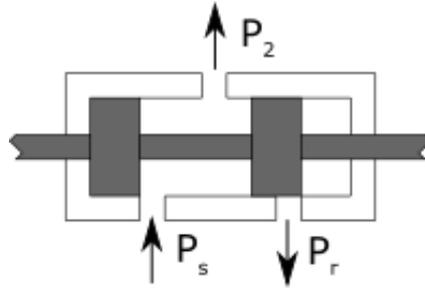
Figure 5-8 Schematic overview of 3-way directional valve
