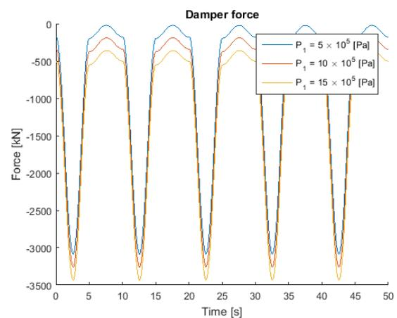
Figure 4-10 Force plot: influence initial pressure in system
