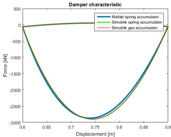
Figure 4-6 Basic damping device characteristic in Force-displacement plot
