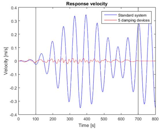
Figure 4-40 Response velocity, excitation frequency close to the natural frequency of the standard system
