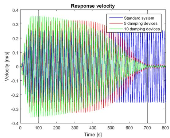
Figure D- 10 Response velocity, different amount of damping devices
