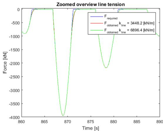
Figure 5-31 Zoomed overview line tension, case 3: different line stiffness
