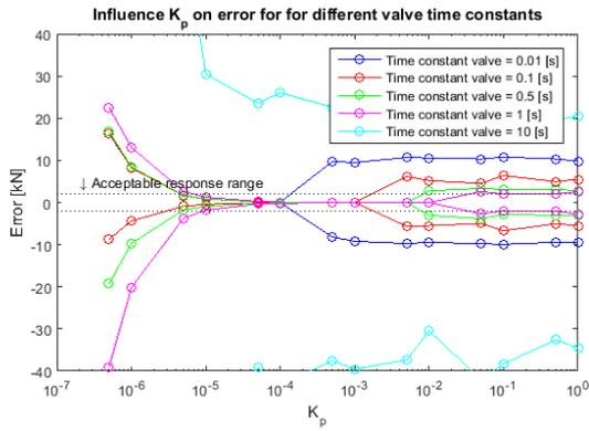
Figure E- 7 Hydraulic system, influence proportional gain,  $F_{amplitude} = 1500$  [kN],  $F_{min} = -100$  [kN]
