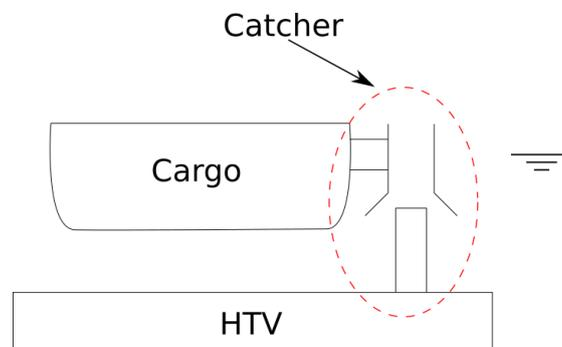
Figure C- 17 Catcher, schematic cross section
