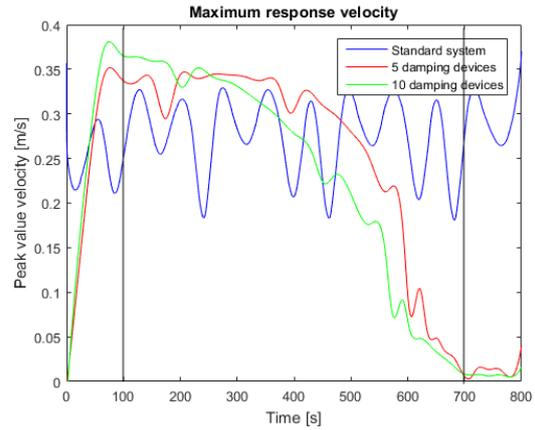
Figure D- 29 Maximum response velocity, irregular force case 3
