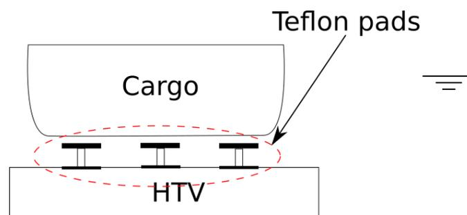
Figure C- 9 Teflon pads, schematic cross section
