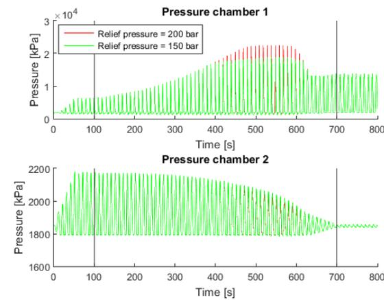
Figure 4-37 Pressure inside the cylinder chambers, different relief pressures (200 bar, 150 bar)
