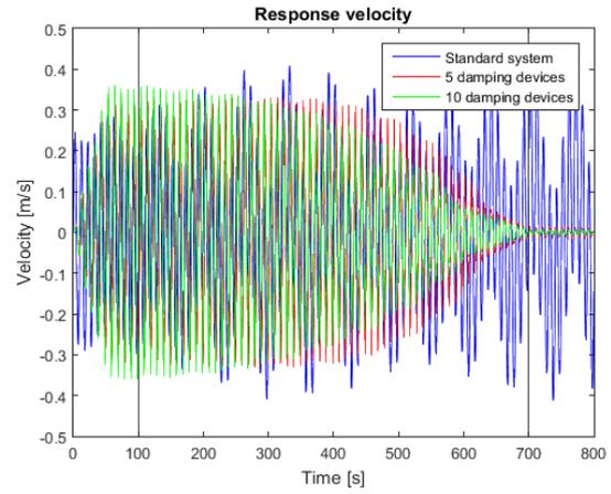
Figure D- 20 Response velocity, irregular force case 2
