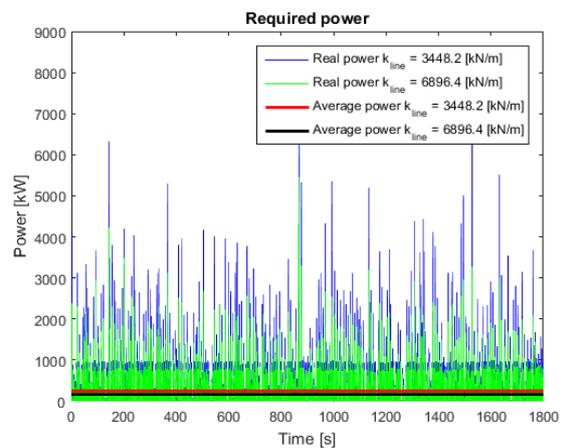
Figure 5-34 Required power, case 3: different line stiffness
