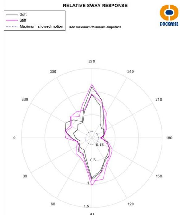
Figure 2-5 Relative sway response in [m]
