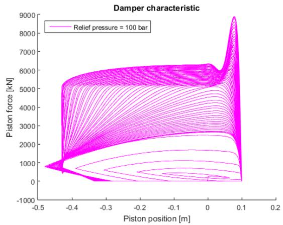
Figure 4-34 Damper characteristic, different relief pressures (100 bar)
