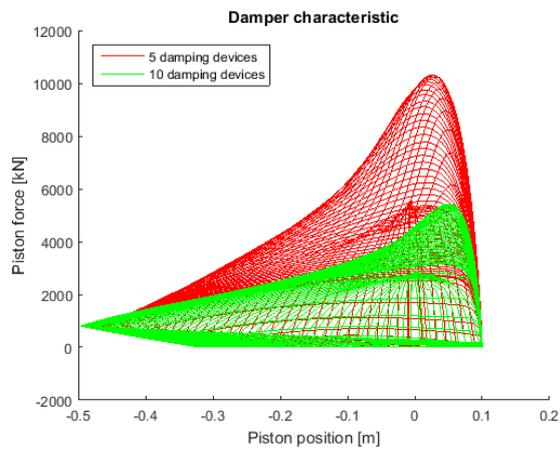
Figure 4-28 Damper characteristic, different amount of damping devices
