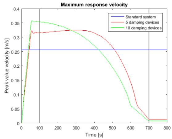
Figure 4-27 Maximum response velocity, different amount of damping devices
