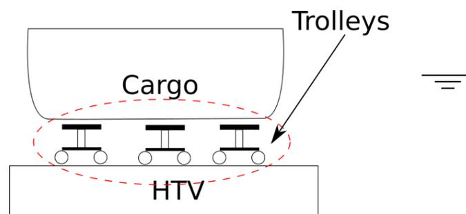
Figure C- 10 Trolleys, schematic cross section
