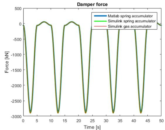
Figure 4-7 Damping force of the basic damping device
