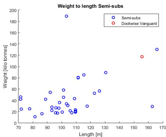
Figure A- 7 Weight to length of semi-sub currently in operation [27]
