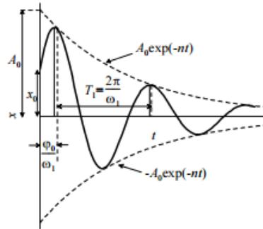
Figure B- 3 Free vibration, underdamped system [11]
