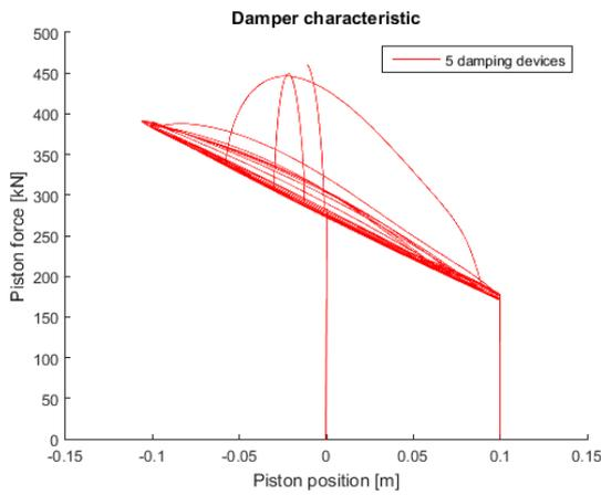
Figure 4-41 Damper characteristic, excitation frequency close to the natural frequency of the standard system
