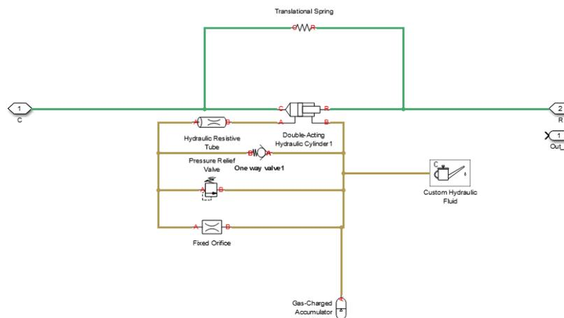
Figure D- 2 SimHydraulics model of the basic damping device
