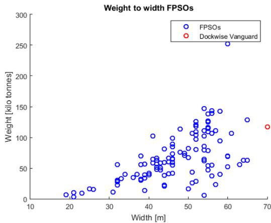
Figure A- 1 Weight to Width of FPSOs in operation [23]
