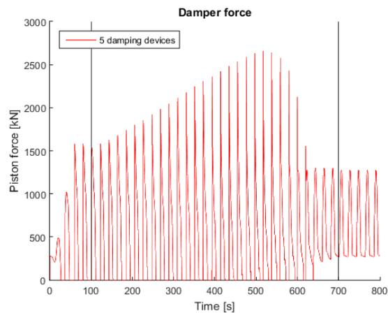
Figure 4-47 Damper force, excitation frequency close to the natural frequency of the new cargo handling system
