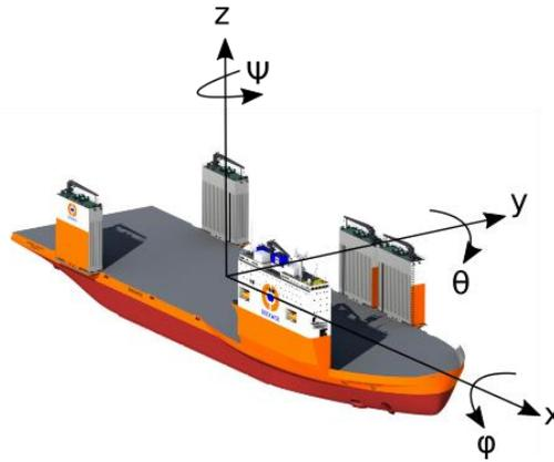
Figure 1-2 Coordinate system ship motions
