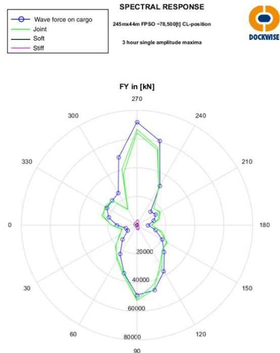
Figure 2-9 Force in sway direction
