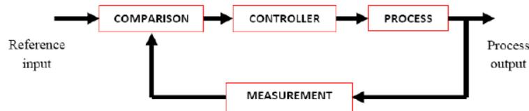
Figure A- 19 Schematic overview closed loop system [6]
