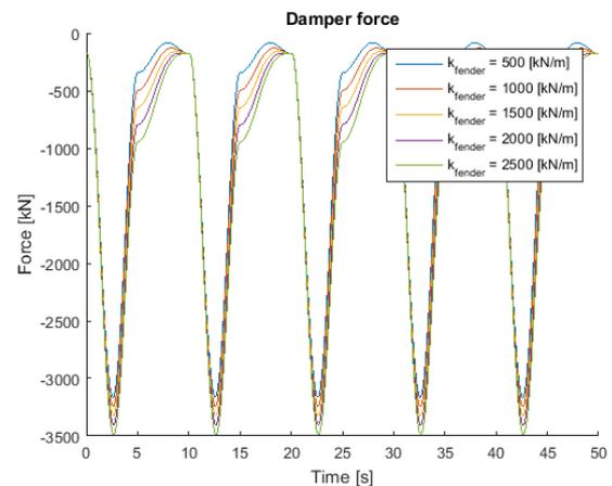
Figure 4-12 Force plot: influence fender stiffness on system
