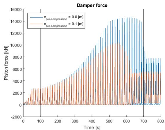
Figure 4-24 Damper force, pre-compression fender
