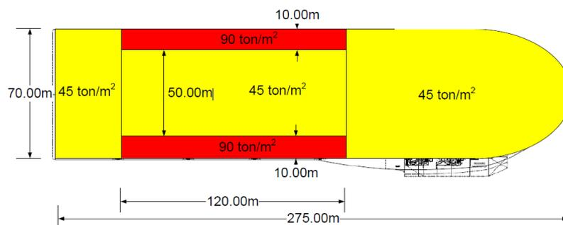
Figure B- 1 Maximum allowable deck load [3]
