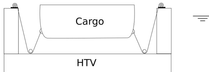
Figure C- 7 Pull the cargo against the deck of the HTV, schematic cross section
