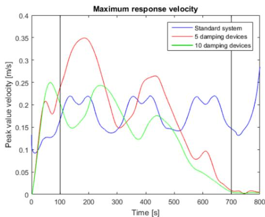
Figure 4-49 Maximum response motion, irregular force case 1
