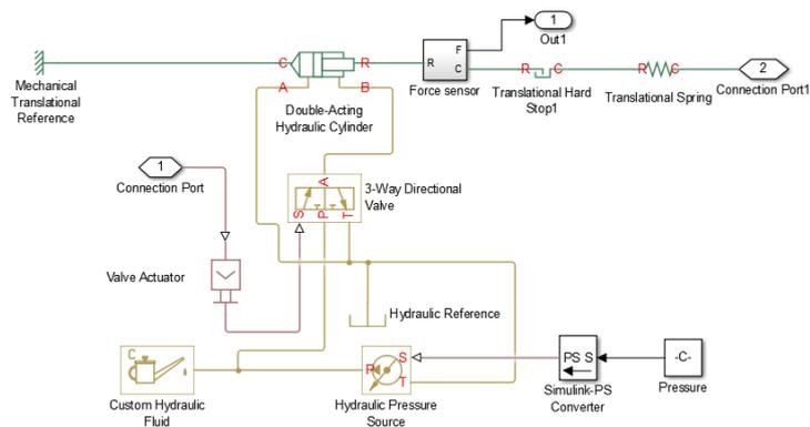
Figure E- 1 SimHydraulics model of the hydraulic actuator
