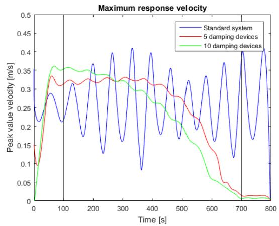
Figure D- 22 Maximum response velocity, irregular force case 2
