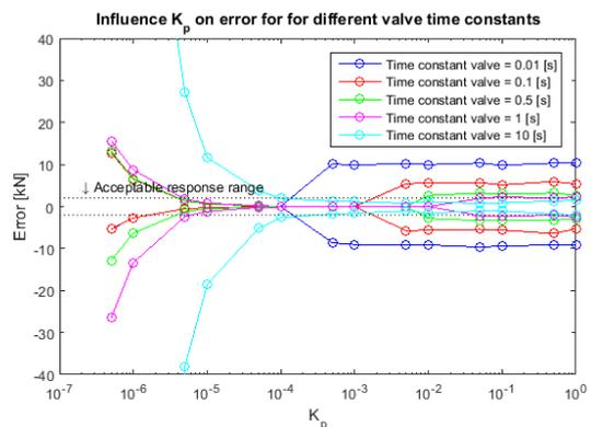
Figure E- 6 Hydraulic system, influence proportional gain,  $F_{amplitude} = 1000$  [kN],  $F_{min} = -100$  [kN]
