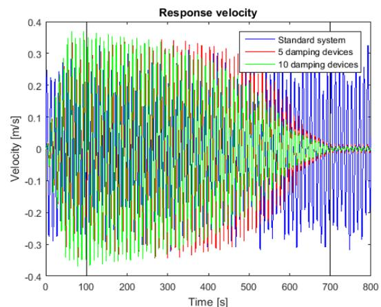
Figure D- 27 Response velocity, irregular force case 3
