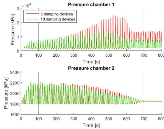
Figure D- 25 Pressure inside the cylinder chambers, irregular force case 2
