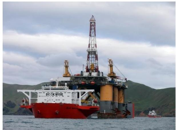
Figure A- 8 Semi-sub on board of the Blue Marlin [24]
