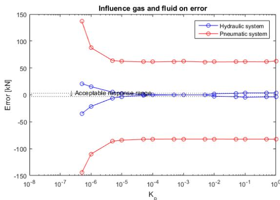
Figure 5-13 Influence of the used fluid on the proportional gain
