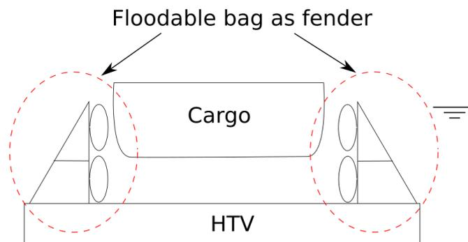
Figure C- 19 Floodable bag as fender, schematic cross section
