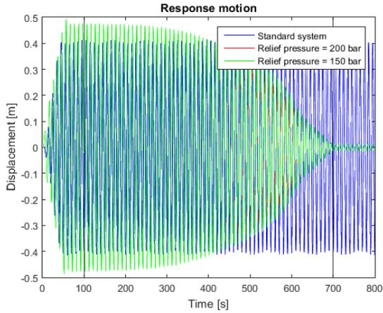
Figure D- 11 Response motion, different relief pressures (200 bar, 150 bar)
