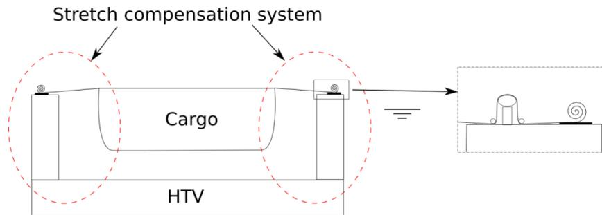
Figure C- 8 Stretch compensation system, schematic cross section
