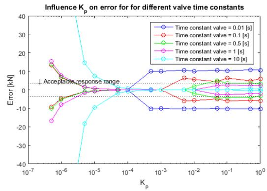
Figure E- 10 Hydraulic system, influence proportional gain,  $F_{amplitude} = 1500$  [kN],  $F_{min} = -500$  [kN]
