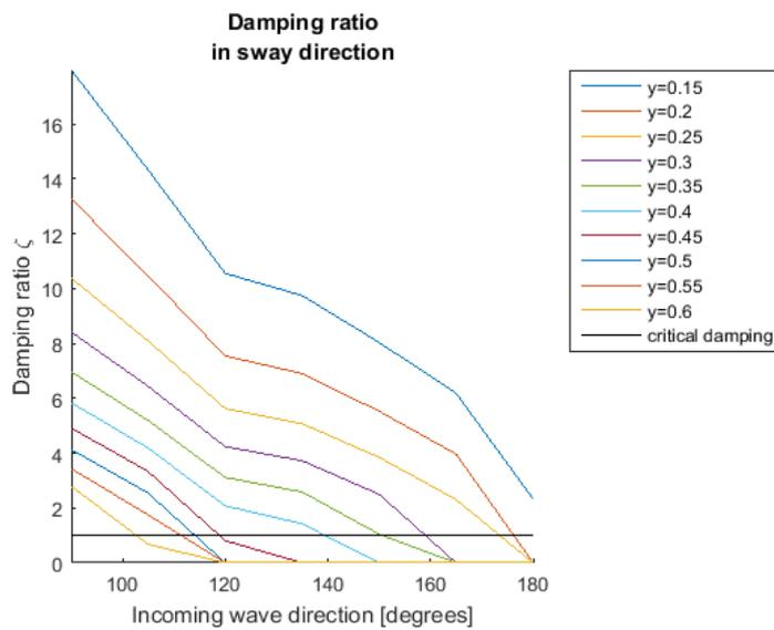
Figure B- 10 Damping ratio in sway direction for different relative motion restrictions
