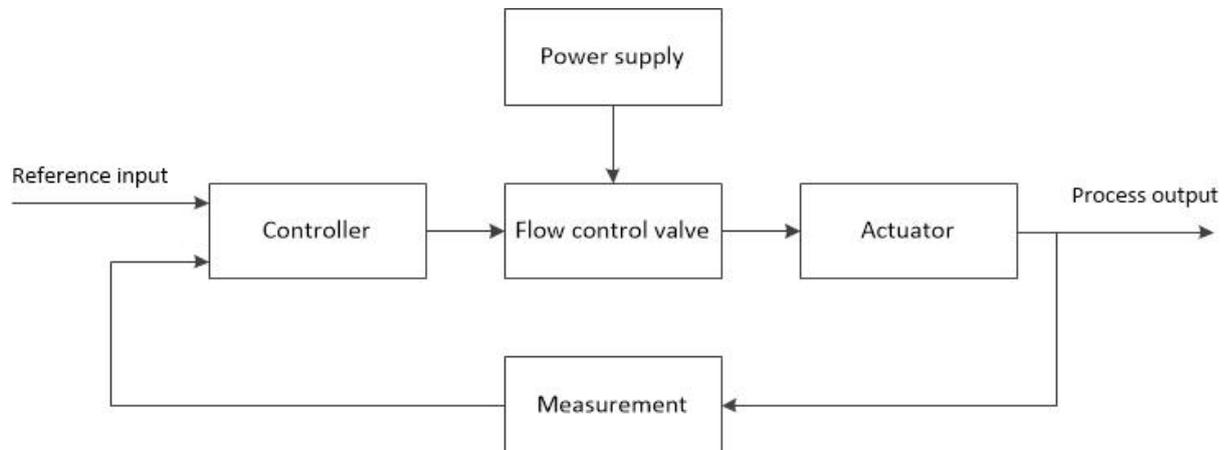
Figure 5-6 Schematic overview control system
