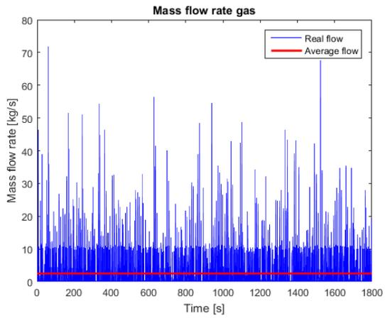
Figure E- 13 Mass flow rate gas, pneumatic actuator 2
