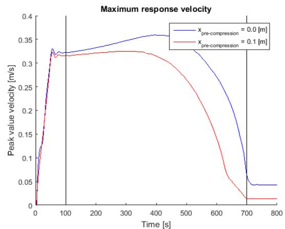
Figure 4-22 Maximum response velocity, pre-compression fender
