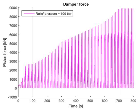
Figure 4-36 Damper force, different relief pressures (100 bar)
