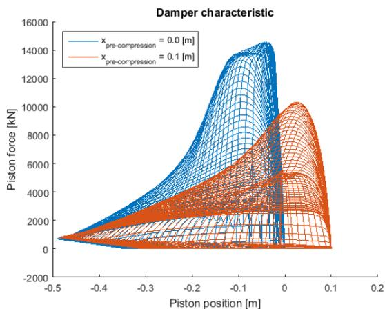
Figure 4-23 Damper characteristic, pre-compression fender
