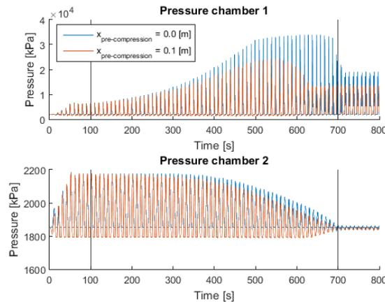
Figure 4-25 Pressure inside the cylinder chambers, pre-compression fender
