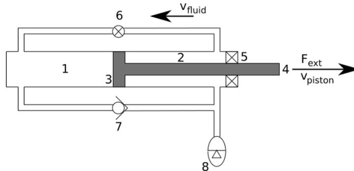
Figure 4-5 Simplified overview basic damping device
