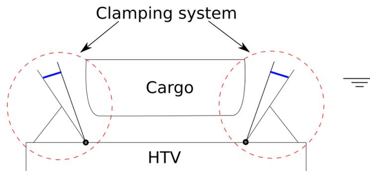
Figure 3-4 Clamping system, schematic cross section
