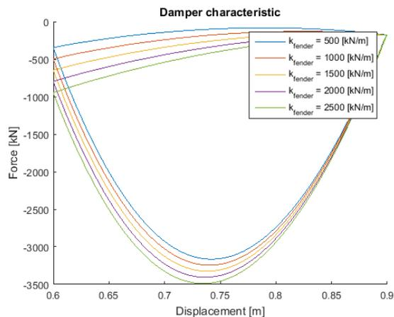
Figure 4-11 Force-displacement plot: influence fender stiffness on system
