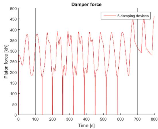
Figure 4-42 Damper force, excitation frequency close to the natural frequency of the standard system
