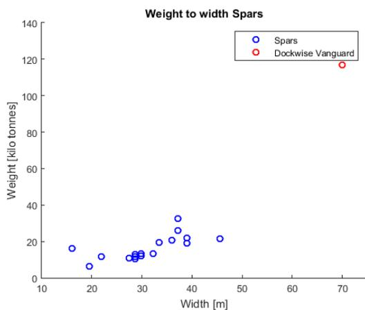
Figure A- 3 Weight to Width of spars in operation [25]
