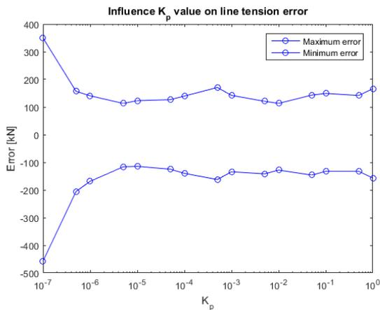
Figure E- 11 Influence proportional gain on line tension error, pneumatic actuator 2
