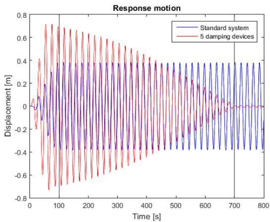
Figure D- 15 Response motion, excitation frequency close to the natural frequency of the new cargo handling system
