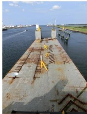
Figure A- 17 Cribbing layout on a vessel deck
