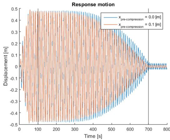
Figure D- 7 Response motion, pre-compression fender
