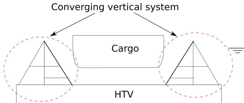
Figure C- 13 Converging vertical system, schematic cross section
