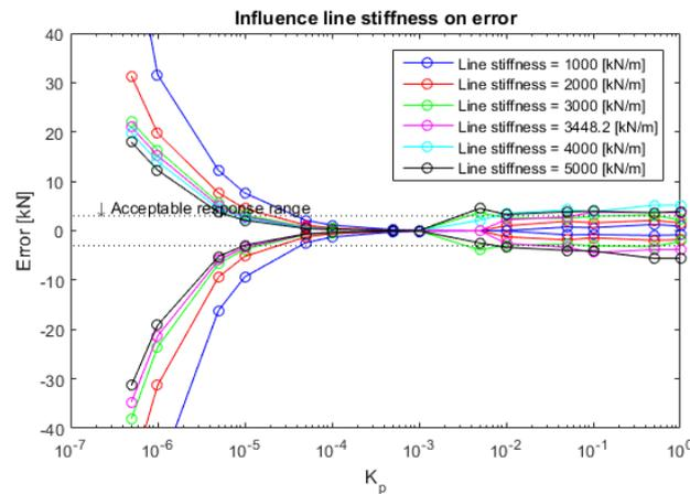
Figure 5-12 Hydraulic system, influence line stiffness on proportional gain
