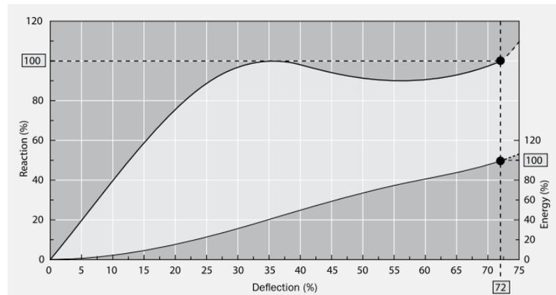
Figure 4-14 Generic curve cone fender [19]
