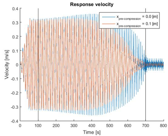
Figure D- 8 Response velocity, pre-compression fender
