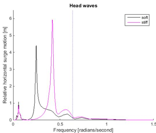
Figure 2-6 Relative surge motion over the frequency
