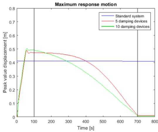
Figure 4-26 Maximum response motion, different amount of damping devices
