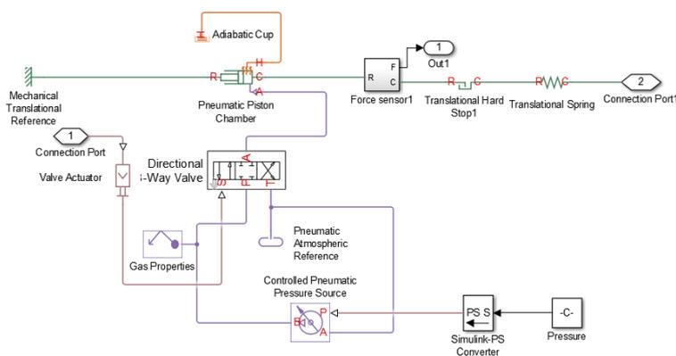
Figure E- 2 SimHydraulics model of the pneumatic actuator
