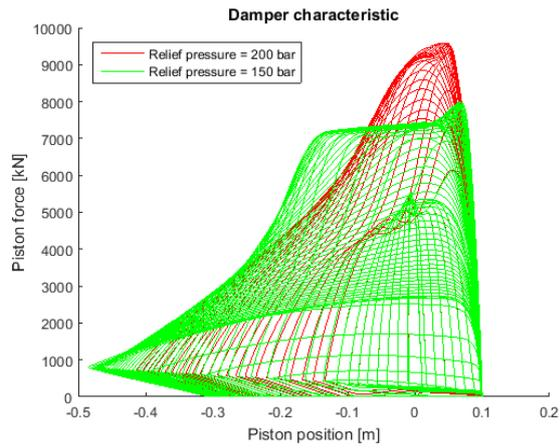
Figure 4-33 Damper characteristic, different relief pressures (200 bar, 150 bar)
