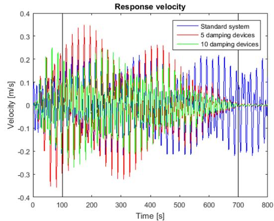
Figure D- 18 Response velocity, irregular force case 1
