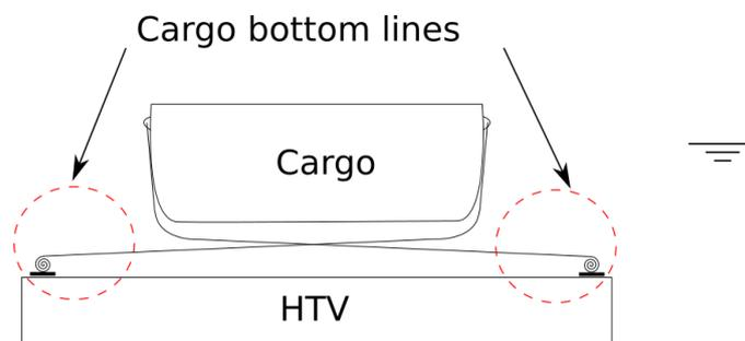
Figure 3-1 Cargo bottom lines, schematic cross section
