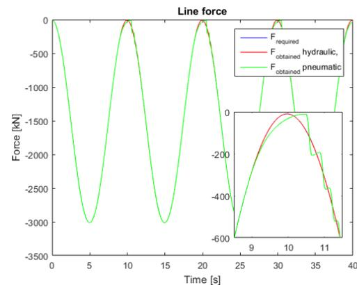
Figure 5-14 Line force of the two different systems
