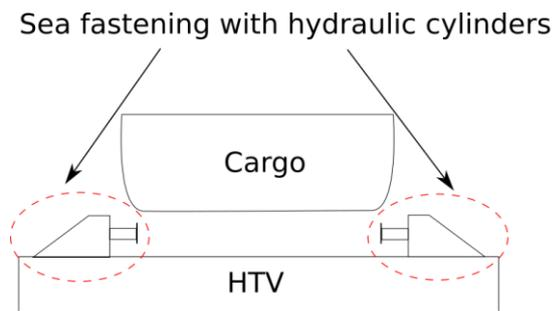
Figure C- 14 First configuration, schematic cross section
