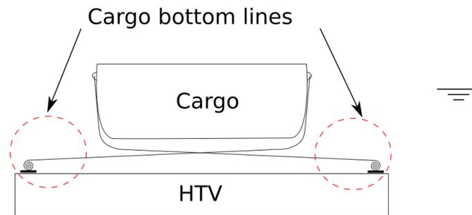
Figure C- 6 Cargo bottom lines, schematic cross section
