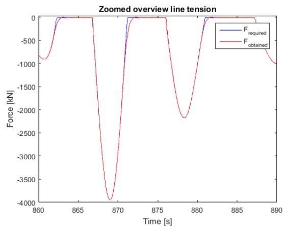
Figure 5-27 Zoomed overview line tension, case 2: pneumatic actuator 1
