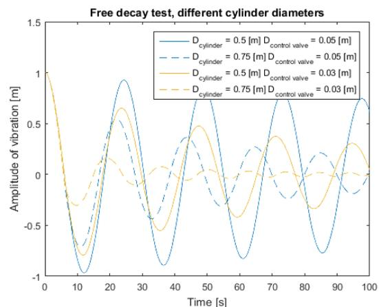
Figure D- 6 Free decay test, different cylinder diameters
