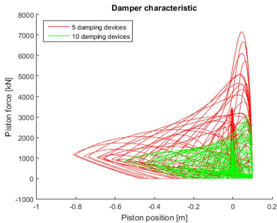
Figure 4-51 Damper characteristic, irregular force case 1
