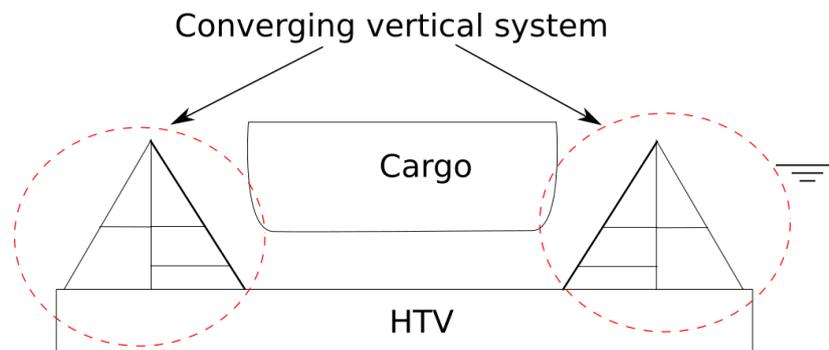
Figure 3-5 Converging vertical system, schematic cross section
