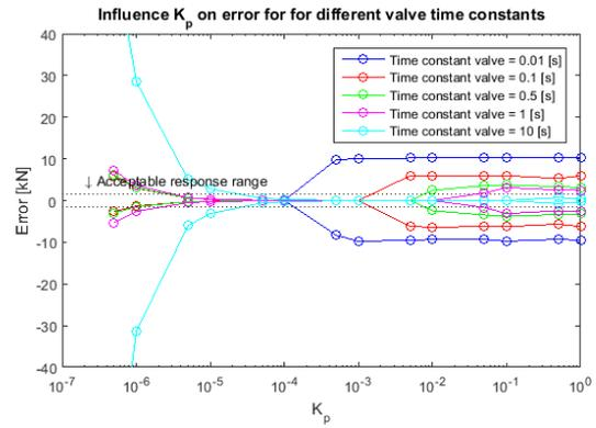
Figure E- 8 Hydraulic system, influence proportional gain,  $F_{amplitude} = 500$  [kN],  $F_{min} = -500$  [kN]
