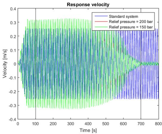
Figure D- 13 Response velocity, different relief pressures (200 bar, 150 bar)
