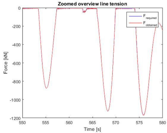
Figure 5-18 Zoomed overview line tension, case 1: hydraulic actuator 1
