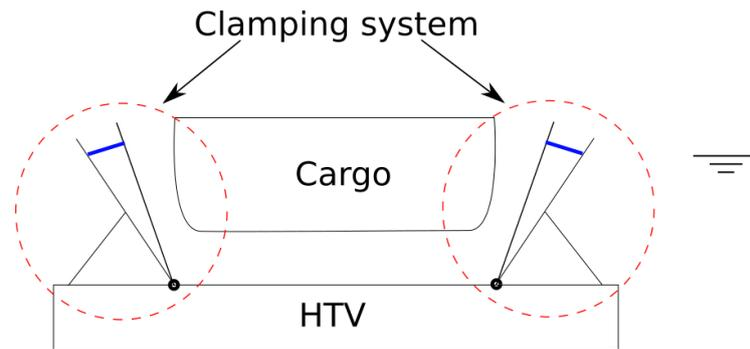
Figure C- 12 Clamping system, schematic cross section
