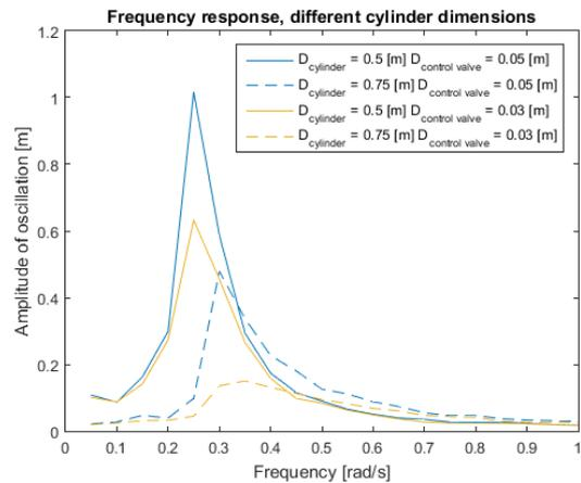
Figure D- 4 Frequency response, different cylinder dimensions
