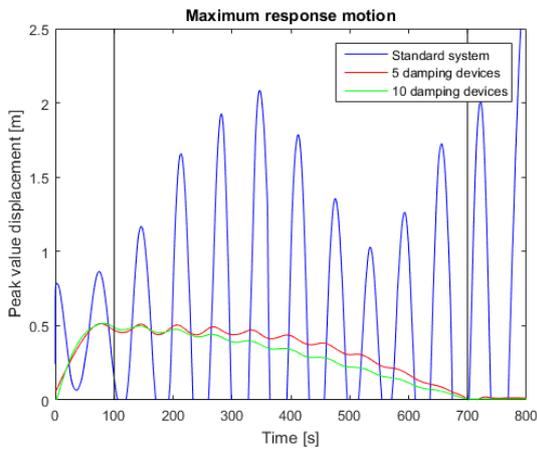
Figure D- 21 Maximum response motion, irregular force case 2
