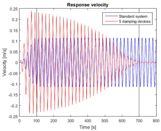
Figure D- 16 Response velocity, excitation frequency close to the natural frequency of the new cargo handling system
