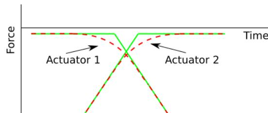
Figure 5-36 Schematic overview smoothening required line tension
