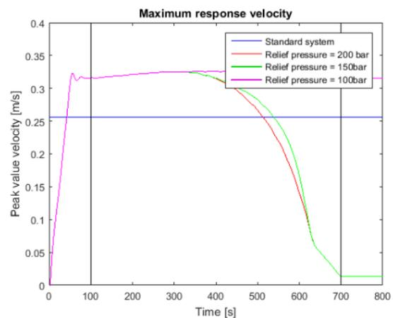
Figure 4-32 Maximum response velocity, different relief pressures
