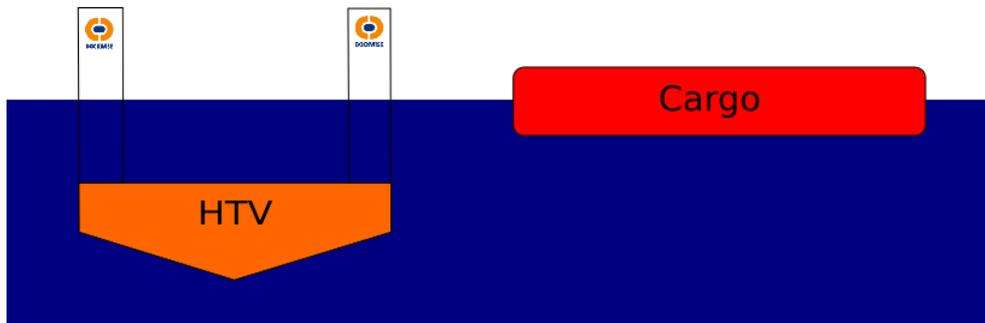
Figure A- 13 Submerging to loading draft
