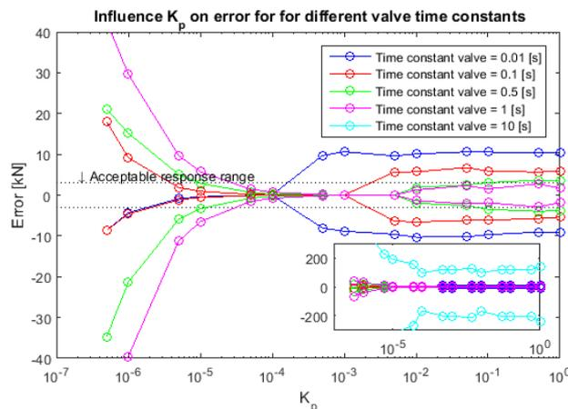
Figure 5-9 Hydraulic system, influence proportional gain,  $F_{amplitude} = 1500$  [kN],  $F_{min} = -10$  [kN]
