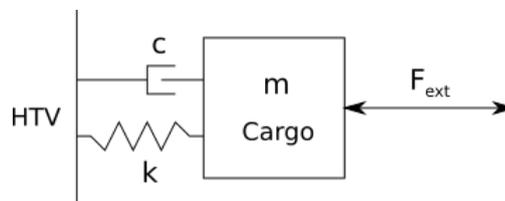
Figure B- 4 MATLAB mass-spring-dashpot model
