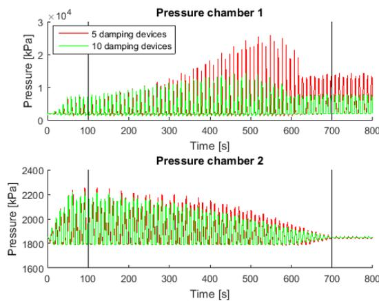
Figure D- 32 Pressure inside the cylinder chambers, irregular force case 3
