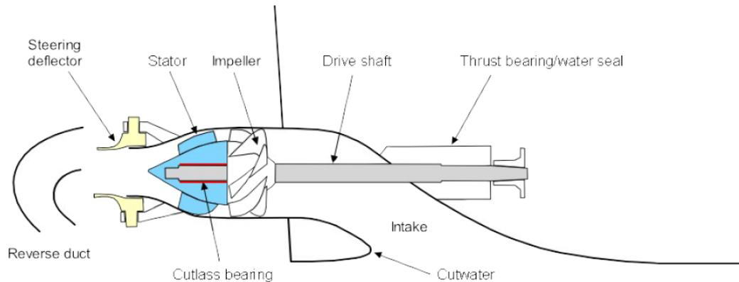
Figure C- 5 Water jet key components [35]
