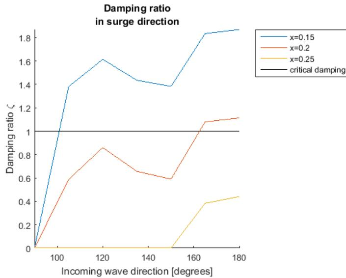
Figure B- 9 Damping ratio in surge direction for different relative motion restrictions
