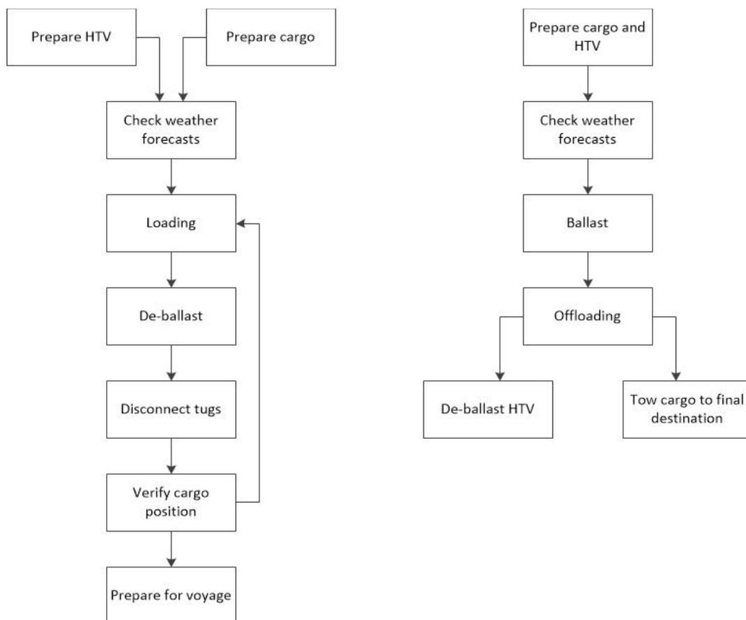
Figure A- 11 Loading and discharge sequence
