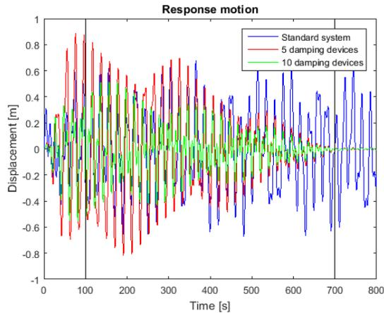
Figure D- 17 Response motion, irregular force case 1
