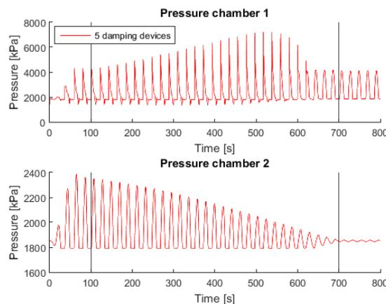
Figure 4-48 Pressure inside the cylinder chambers, excitation frequency close to the natural frequency of the new cargo handling system
