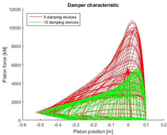
Figure D- 23 Damper characteristic, irregular force case 2
