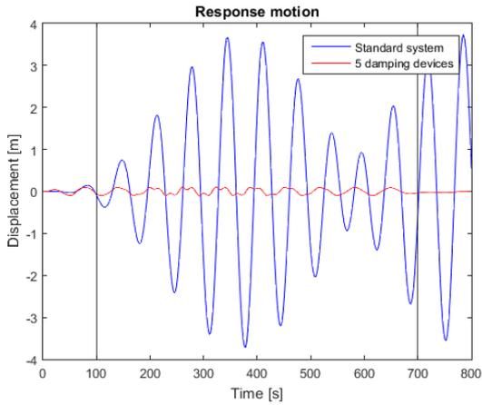
Figure 4-39 Response motion, excitation frequency close to the natural frequency of the standard system
