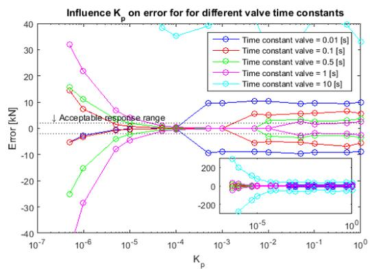
Figure E- 4 Hydraulic system, influence proportional gain,  $F_{amplitude} = 1000$  [kN],  $F_{min} = -10$  [kN]
