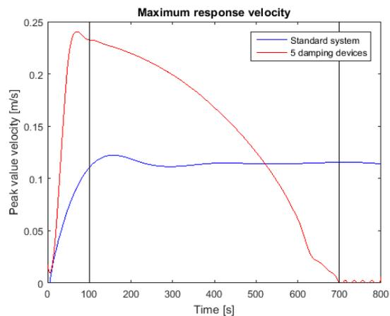
Figure 4-44 Maximum response motion, excitation frequency close to the natural frequency of the new cargo handling system
