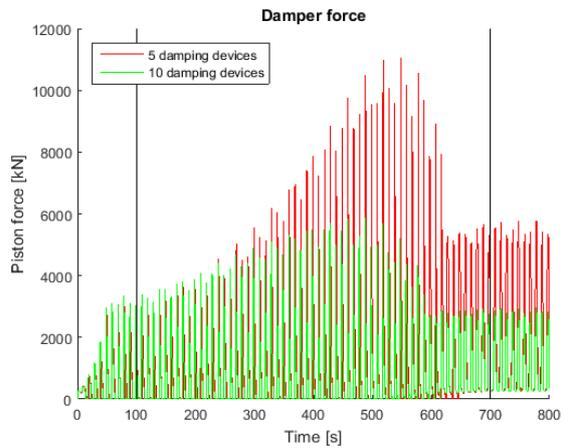
Figure D- 31 Damper force, irregular force case 3
