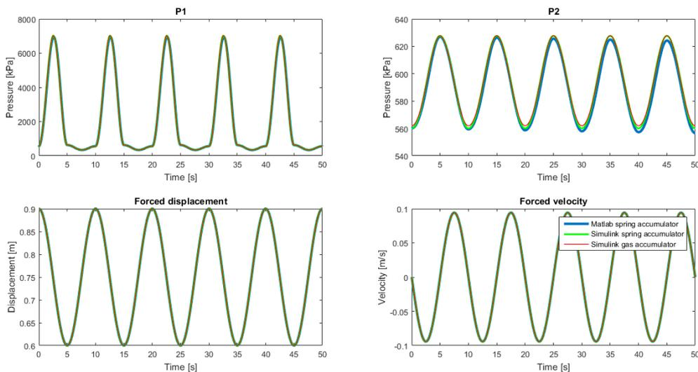
Figure 4-8 Pressures inside the cylinder chambers and piston displacement and velocity of the basic damping device
