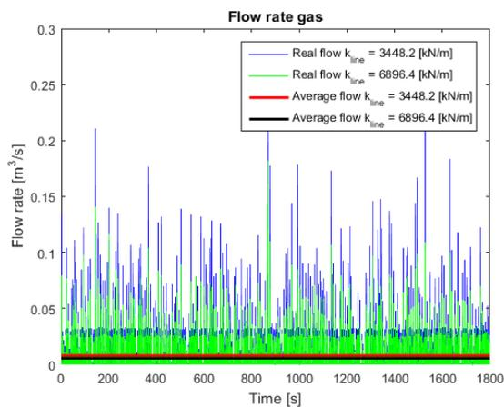
Figure 5-33 Flow rate gas, case 3: different line stiffness
