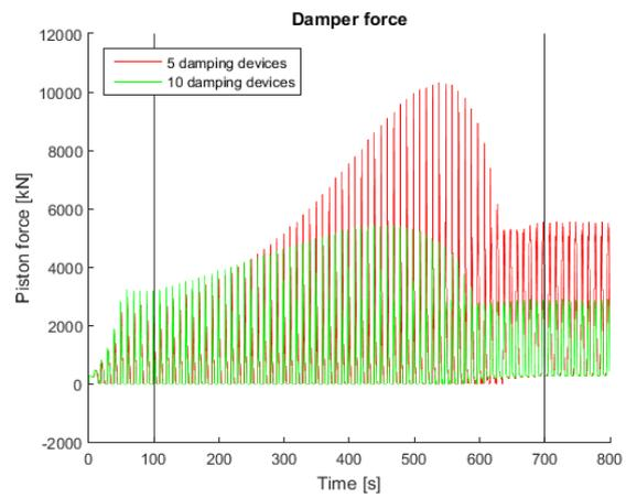
Figure 4-29 Damper force, different amount of damping devices
