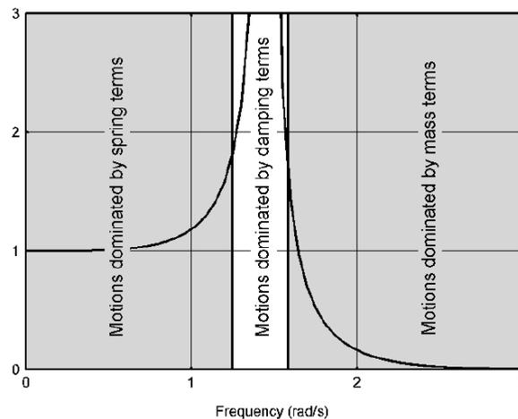
Figure 2-10 Frequency areas with respect to motional behaviour [4]
