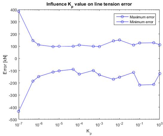
Figure 5-17 Influence proportional gain on line tension error, case 1: hydraulic actuator 1
