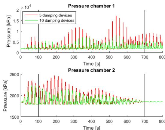
Figure 4-53 Pressure inside the cylinder chambers, irregular force case 1
