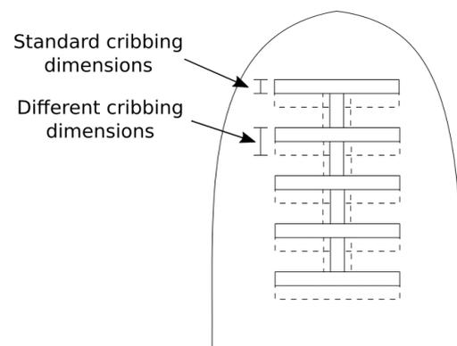
Figure C- 23 Change the cribbing dimensions, schematic top view
