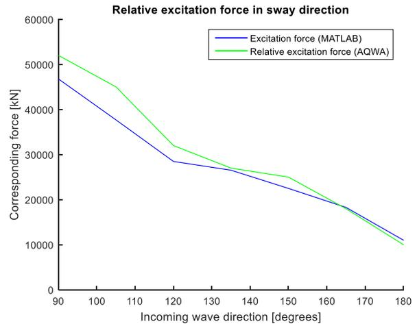
Figure B- 8 Relative excitation force in sway direction
