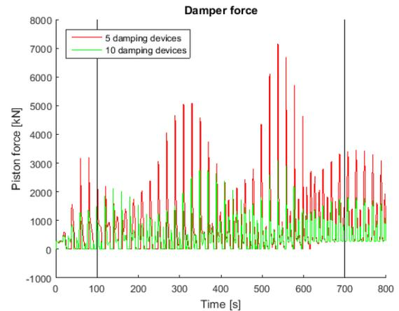
Figure 4-52 Damper force, irregular force case 1
