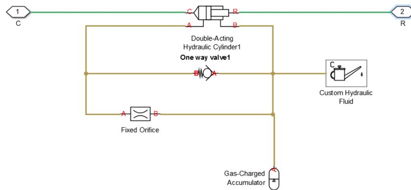
Figure D- 1 SimHydraulics model of the basic damping device
