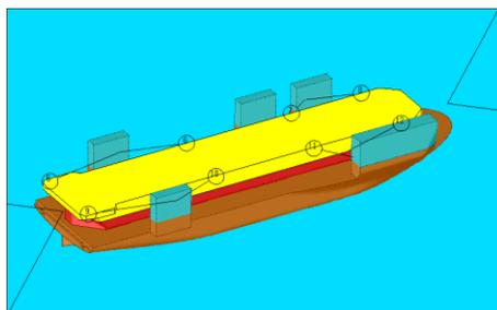
Figure 2-3 Mooring configuration of present cargo handling system
