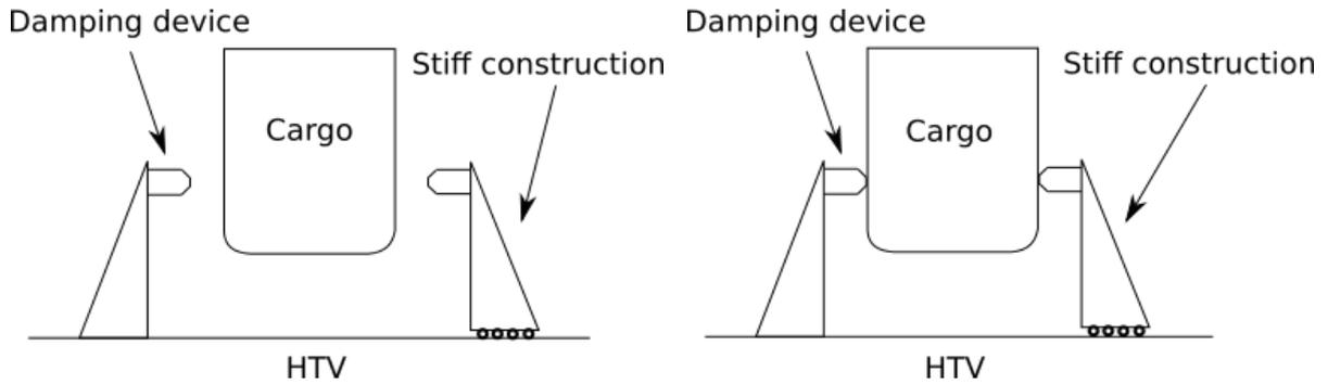
Figure 4-1 Clamping system phase 1
