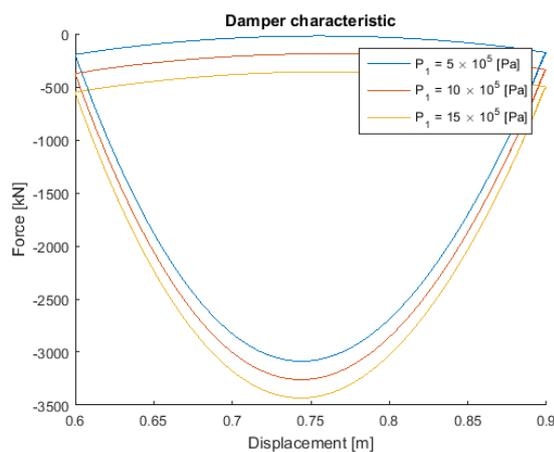
Figure 4-9 Force-displacement plot: influence initial pressure in system
