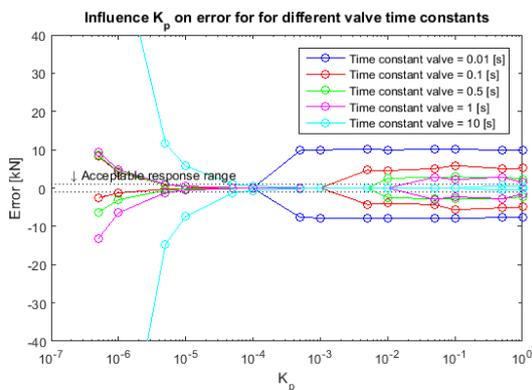
Figure E- 5 Hydraulic system, influence proportional gain,  $F_{amplitude} = 500$  [kN],  $F_{min} = -100$  [kN]
