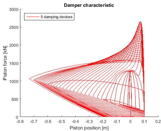
Figure 4-46 Damper characteristic, excitation frequency close to the natural frequency of the new cargo handling system
