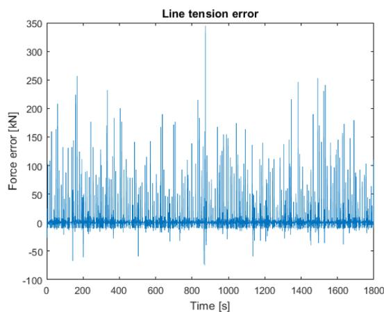
Figure 5-28 Line tension error, case 2: pneumatic actuator 1
