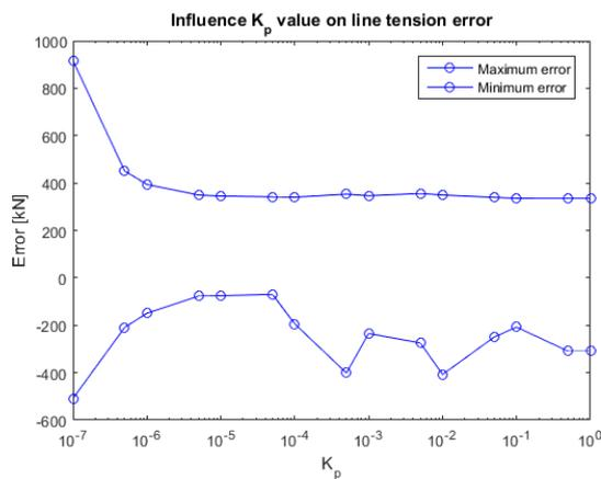
Figure 5-26 Influence proportional gain on line tension error, case 2: pneumatic actuator 1
