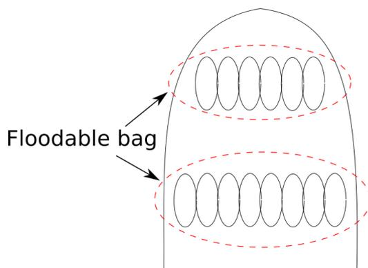
Figure C- 22 Floodable bags as support system, schematic top view
