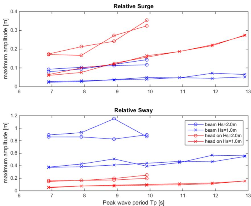
Figure B- 2 Maximum amplitudes for different wave characteristics
