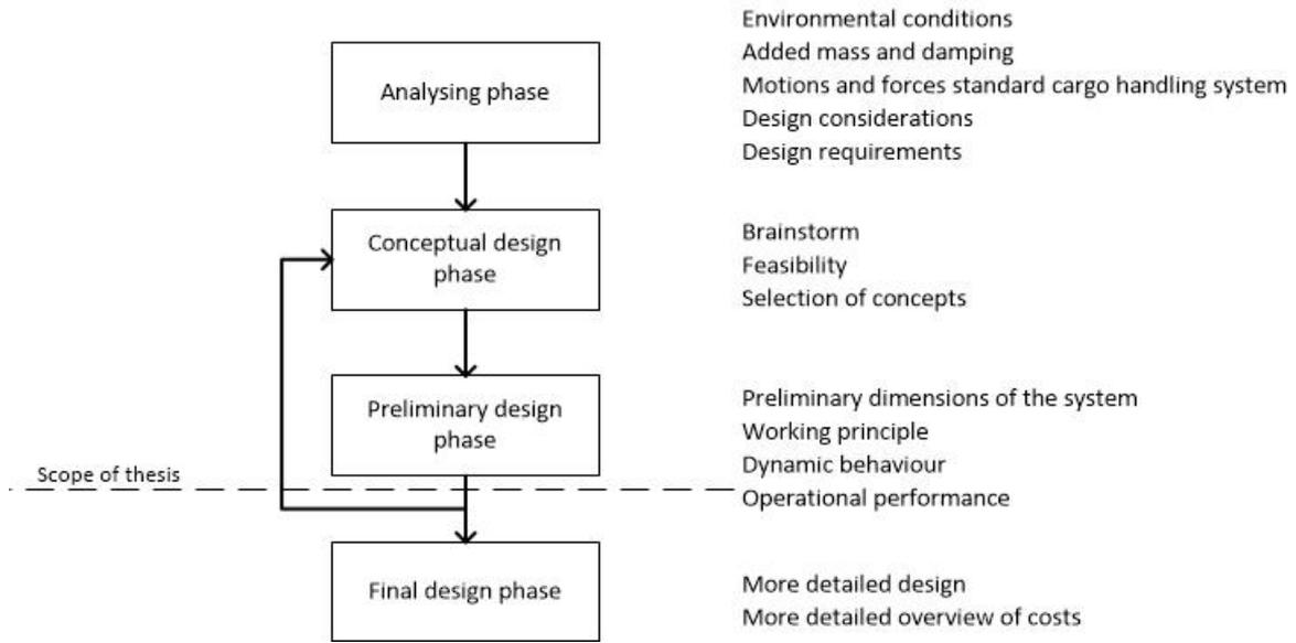
Figure 1-3 Design trajectory
