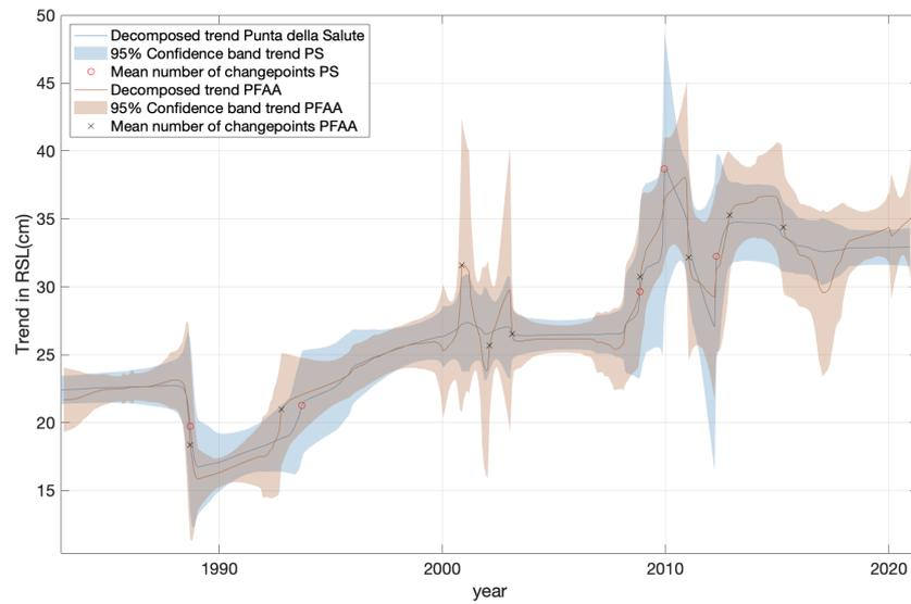
Figure A.2: Changepoints and the decomposed trend and its confidence band of the Punta della Salute and Piattaforma Acqua Alta time-series
