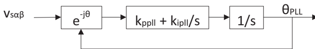
FIGURE 9.33 Block diagram of small signal model of synchronous rotational frame phase locked loop (PLL).
