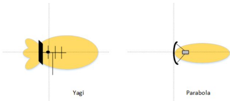
Figure 11: The radiation patterns of a Yagi and parabola antenna [19].
