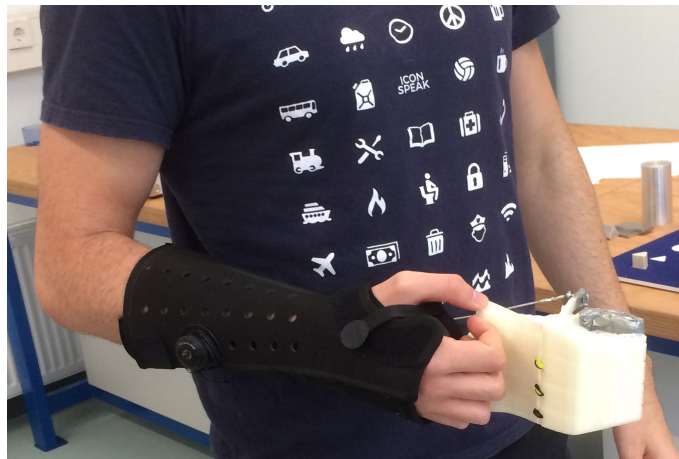
Figure 5.7: Healthy subject wearing the simulator and the prosthetic hand for the user testing
