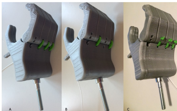
Figure 5.4: Different combinations of elastic bends: A three double elastics, B two double elastics, c three single elastics
