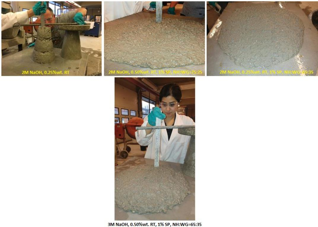
Figure 22: Workability [slump] tests
