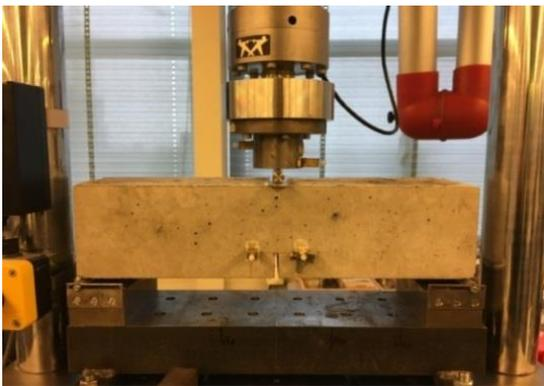
Figure 30: Flexural strength test setup
