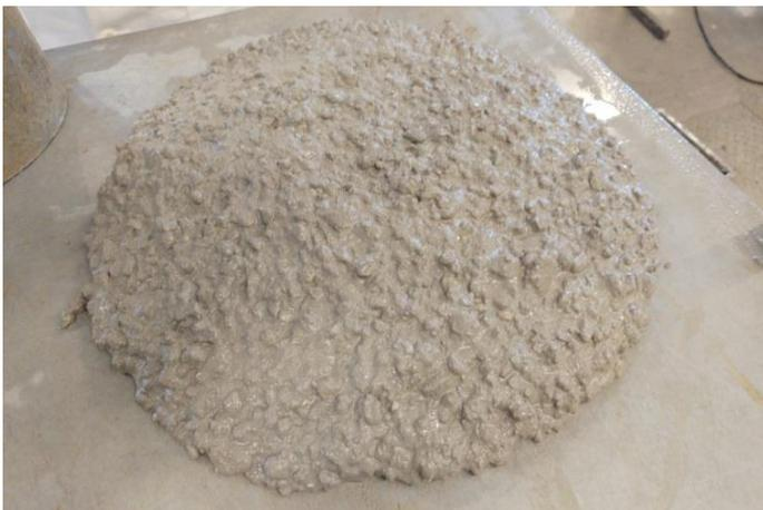
Figure 27: Slump test of optimized concrete mixture
