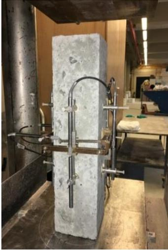
Figure 32: E-modulus test setup
