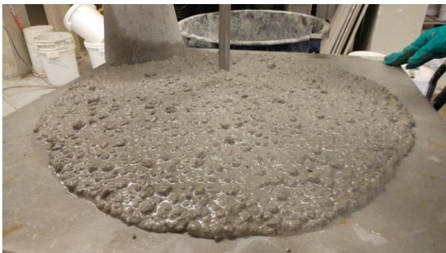
Figure 24: Slump test of mixture III (4M NaOH, 0.5%wt. RT)
