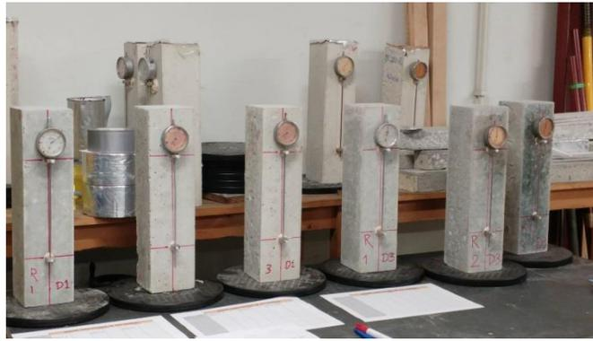
Figure 34: Drying shrinkage test setup
