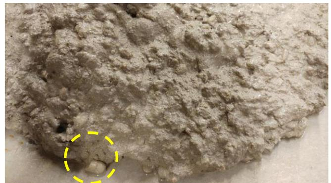
Figure 25: Segregation during the slump test of mixture IV (4M NaOH, 0.75%wt. RT)
