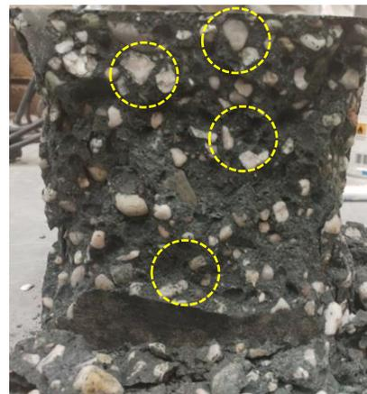
Figure 28: Dotted yellow circles indicate good bonding between matrix and aggregates in the optimized mixture
