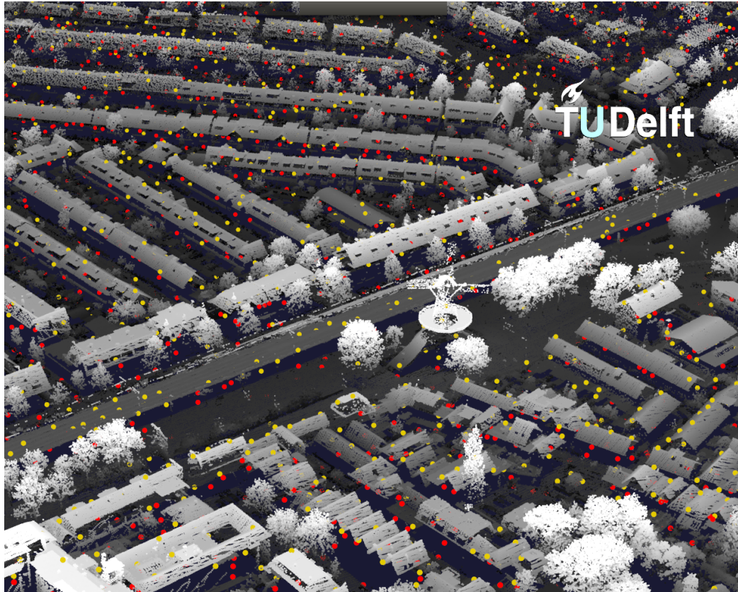
Figure 17: TerraSAR-X PSI results of Delft shown along AHN2 in a AHN2 viewer. The coloured dots are point scatterers, the red are from the descending pass, from a stack of 72 acquisitions; the yellow from the ascending pass, using 68 acquisitions. The descending pass looks from the lower right with an incidence angle of 24^\circ , the ascending from the upper left with an incidence angle of 39^\circ . The area is the northern part of the Spoorzone, around the windmill De Roos. Reflections from roofs, ground-wall corners and train rails can be identified.
