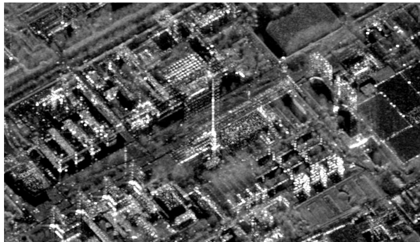
Figure 2: Radar image showing part of Delft University of Technology. The radar looks from the top, so the bottom of the buildings is lower in the image than the top, as you would expect in a optical picture. Shadows can be clearly seen below a number of buildings. The most prominent building, the 22 story EWI building in the centre of the image, is overlayed on top of the Mekelpark and the civil engineering building and its shadow. Note that you're looking at the 'back' side of the buildings, the side that is pointing away or up, as the radar observes from the top. Especially interesting in this view is the lack of shadow of the EWI building. While it is by far the highest building there is no shadow at all. This is because the building acts as a mirror, and the terrain and building at the radar side of the building are seen through this mirror. The signal has to travel a longer way, and as such it ends up further away in range in the image. This image is created by averaging 72 images taken between 2009 and 2011 by the TerraSAR-X satellite. It is taken with a wavelength of 16 mm, a ground resolution of 3 \times 3 m, and an incidence angle of 24^\circ .
