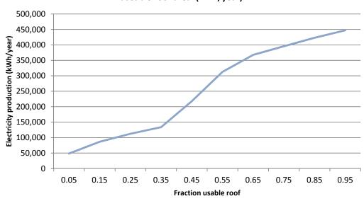
Figure 38 Electricity production by solar panels in neighbourhood usable roof area (kWh/year)
