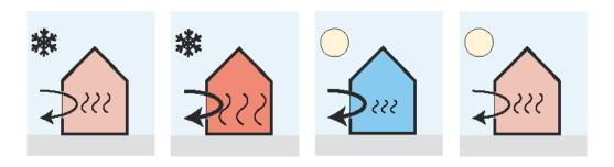
Figure 51: Concept heat recovery ventilation. The heat recovery is regulated according to the indoor and outdoor climate.
