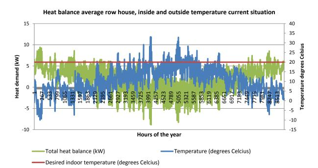
Figure 109 Heat balance average row house, inside and outside temperature current situation
