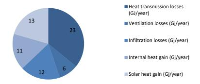
Figure 43 Yearly heat balance apartment flat type 1 current situation
