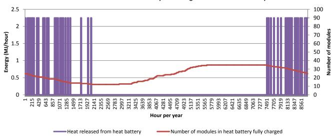
Figure 64 Use of heat modules of heat battery for average row house over whole year
