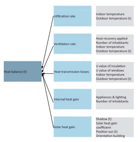
Figure 42 Heat balance model
