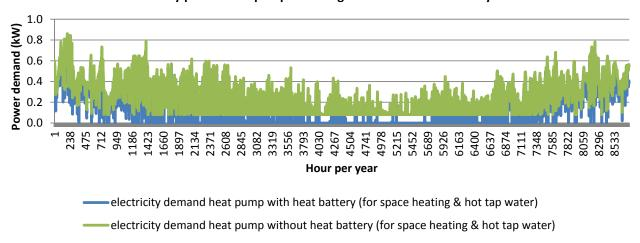
Figure 119 Electricity profile heat pump of average row house over whole year
