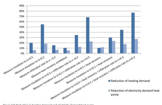
Figure 116 Reduction in heating demand and electricity demand heat pump
