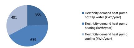
Figure 56 Annual electricity demand heat pump average apartment flat type 1 improved situation
