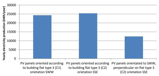
Figure 35 Yearly electricity production by solar panels for different orientations on flat type 3
