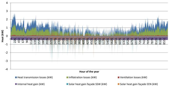
Figure 47 Losses and gains heat balance average row house improved situation
