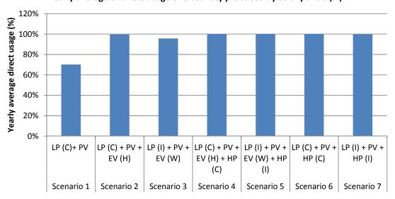
Figure 107 Direct usage of electricity produced by solar panels
