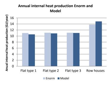
Figure 88 Annual internal heat production Enorm and Model
