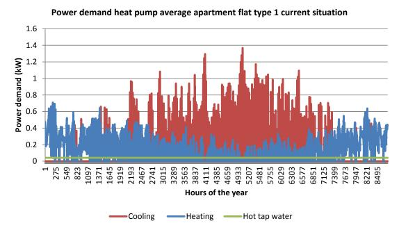
Figure 117 Power demand heat pump average apartment flat type 1 current situation
