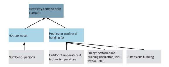
Figure 39 Concept electricity demand heat pump
