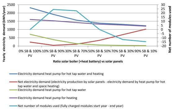
Figure 69 Yearly electricity demand heat pump (solar boiler & heat battery vs solar panels
