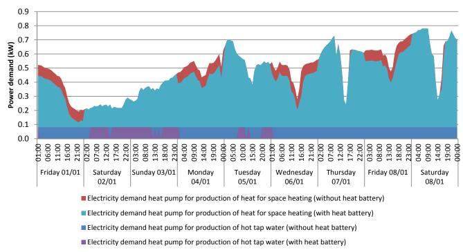
Figure 66 Electricity profile heat pump with and without heat battery for average row house in winter week
