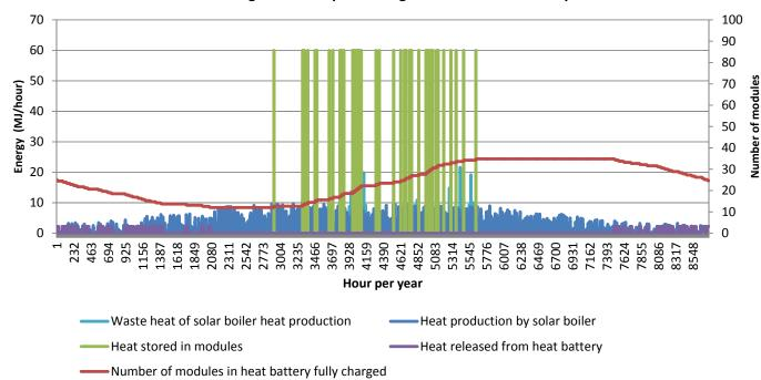
Figure 65 Functioning heat battery for average row house over whole year
