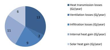
Figure 45 Yearly heat balance apartment flat type 1 improved situation
