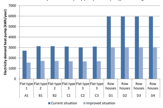
Figure 115 Annual electricity demand heat pump per apartment per type of building
