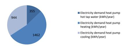
Figure 54 Annual electricity demand heat pump average apartment flat type 1 current situation
