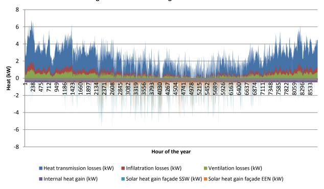
Figure 48 Losses and gains heat balance average row house current situation
