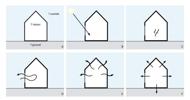
Figure 41 Concept of heat balance
