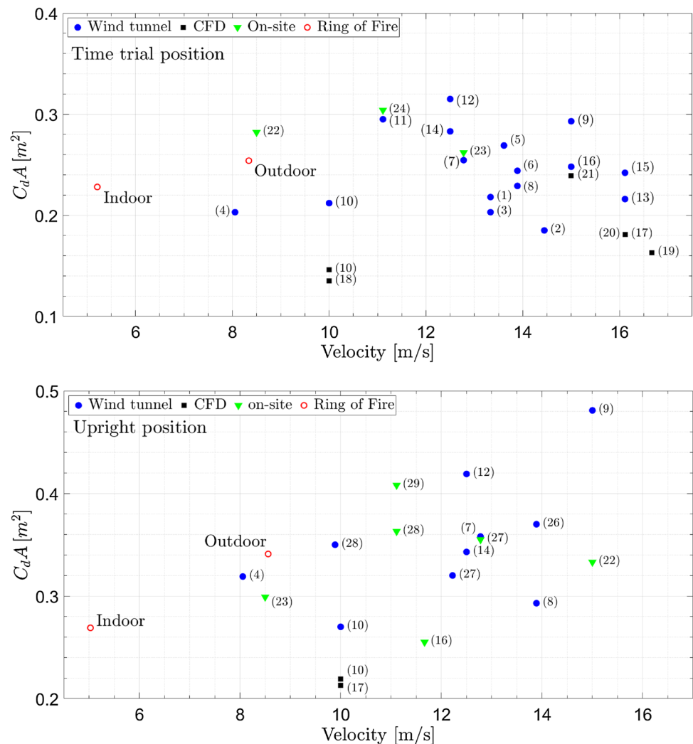
Fig. 14 Comparison of drag area of a cyclist in time-trial position (top) and in upright position (bottom) measured with different measurement techniques at different velocities. 1 Kyle (1991), 2 Hill (1993), 3 Broker and Kyle (1995), 4 Zdravkovic et al. (1996), 5 Martin et al. (1998), 6 Padilla et al. (2000), 7 Jeukendrup and Martin (2001), 8 Gibertini and Grassi (2008), 9 Garcia-Lopez et al. (2008), 10 Defraeye et al. (2010), 11 Underwood et al. (2011), 12 Chowdhury and Alam (2012), 13 Crouch et al. (2014), 14 Barry et al. (2015), 15 Crouch et al. (2016), 16 Blocken et al. (2016), 18 Griffith et al. (2012), 19 Blocken et al. (2013), 20 Defraeye et al. (2014), 21 Griffith et al. (2014), 23 Grappe et al. (1997), 24 Candau et al. (1999), 25 Peterman et al. (2015), 26 Nonweiler (1958), 27 Kyle and Burke (1984), 28 Fintelman et al. (2014), 29 Capelli et al. (1993), 30 de Groot et al. (1995), 31 Lim et al. (2011)
