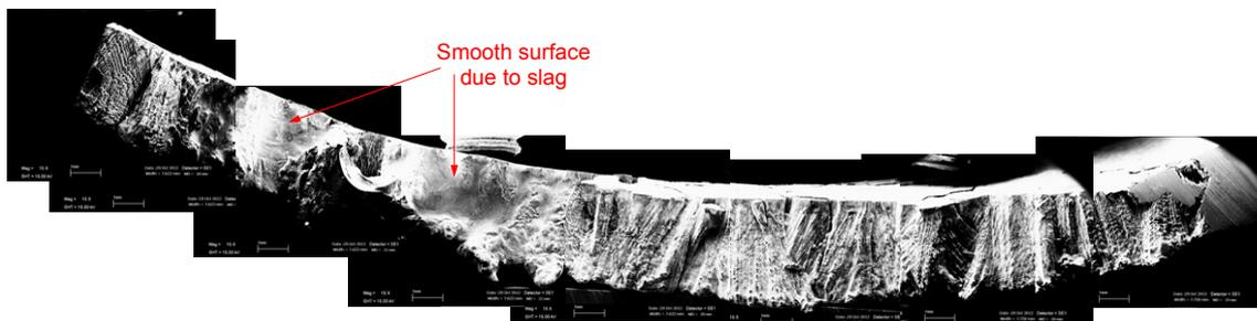
Figure 6.14. Fracture surface of crack sample 2B
