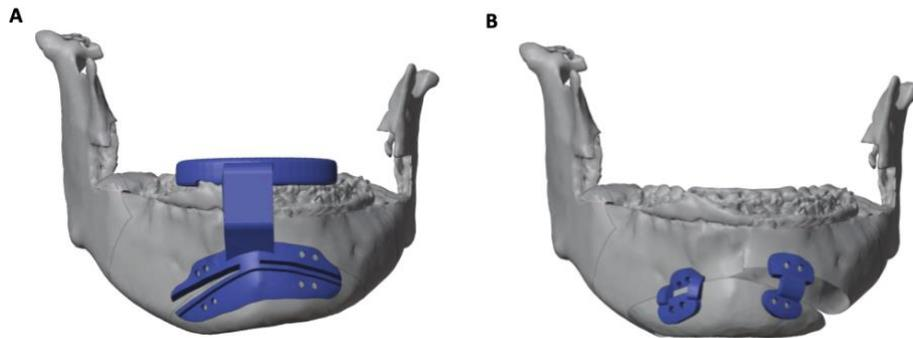
Figure 10 Intended design of the patient-specific guidance system. A) The cutting guide (blue) is supported by the dentition and bone (grey). Screw holes are drilled and used for fixation during the osteotomy. B) The repositioning guides (blue) are positioned using the screw holes from the cutting guide.
