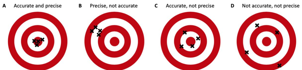
*Figure 4 Difference between accuracy and precision. Bull's eye of the target represents the ground truth. The black crosses signify individual test results. A) Accurate and precise, B) Precise but not accurate, C) Accurate but not precise, D) not accurate and not precise.*
