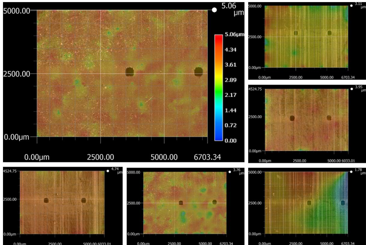
In the right top corner of every sub-figure the maximum surface roughness of the valve seat of that particular microvalve base is shown. The estimated surface roughness is  $3.69 \pm 1.32 \mu m$ .
