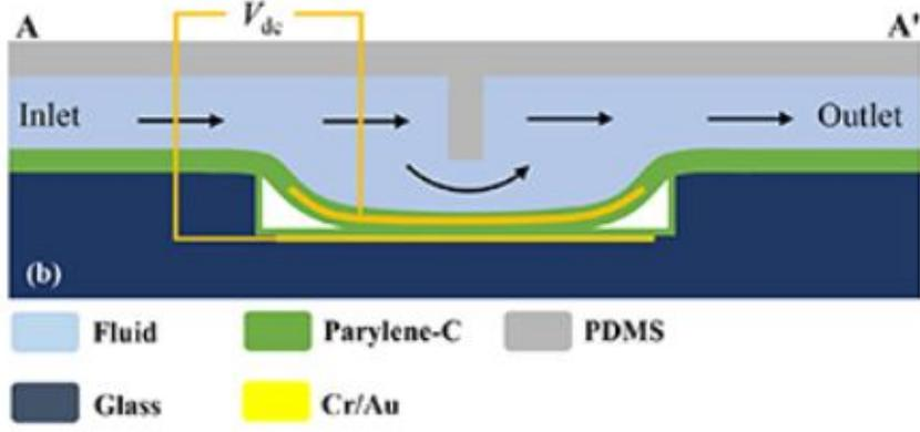
Figure 4: NC electrostatic actuated microvalve [35]
