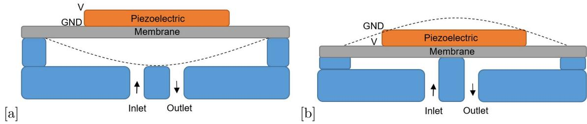
Figure 19: (a) NO piezoelectric actuated microvalve configuration (b) NC piezoelectric actuated microvalve configuration
