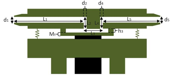
Figure 8: Cross-section of the microvalve base. The design parameters are: Inlet channel length ( $L_1$ ), Inlet channel diameter ( $d_1$ ), Chamber inlet length ( $L_2$ ), Chamber inlet diameter ( $d_2$ ), Chamber length ( $L_3$ ), Valving Chamber height ( $h_3$ ), Chamber outlet length ( $L_4$ ), Chamber outlet diameter ( $d_4$ ), Outlet channel length ( $L_5$ ), Outlet channel diameter ( $d_5$ ), Membrane thickness ( $M_t$ ).
