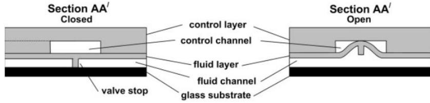
Figure 12: NC pneumatic microvalve [48]
