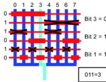
Figure 13: Schematic image of the Complementary Binary Multiplexer, where the blue lines represent the flow channels and the red lines the control lines. At the intersection of the control lines and the flow lines the bigger rectangular red blocks represents the locations of the microvalves. In this example flow channel 3 is selected forward. [17][18]
