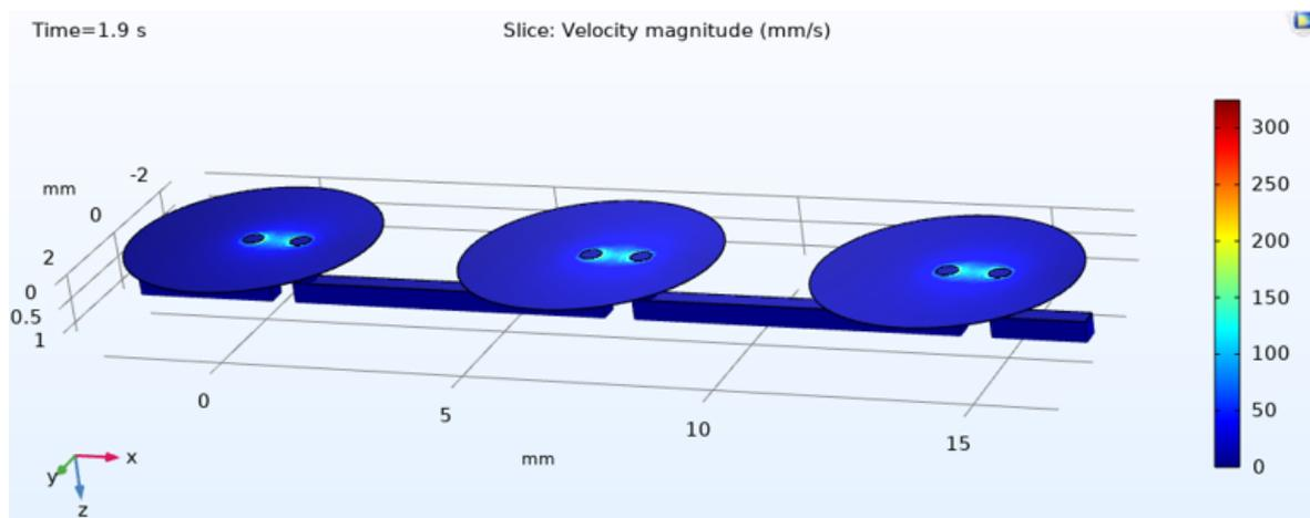
Figure 22: Flow simulation of three NO- microvalves in series
