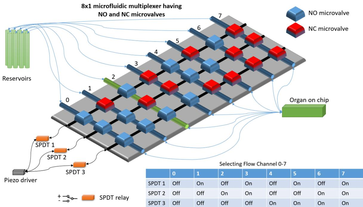
Figure 20: Integration of the piezoelectric binary multiplexer in the OOCs platform
