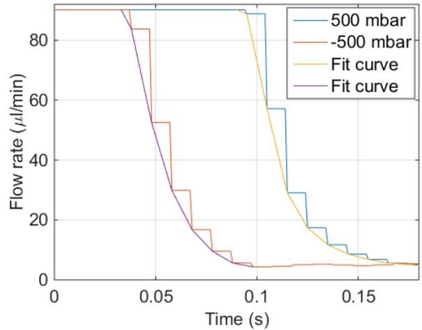
Figure 21: Closing time of the microvalve at 500 and -500 mbar. A fit curve is used to make a smooth closing curve. The closing times are  $45.0 \pm 5.8$  ms (500 mbar) and  $47.8 \pm 6.8$  ms (-500 mbar).
