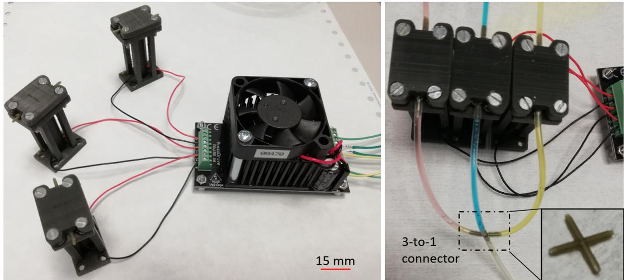
To create a 3-to-1 fluid selector the outputs of the three microvalves are connected by tubings to a 3-to-1 connector. The 3-to-1 connector has 1 output in which the selected fluid is channeled forward. A detailed view of the 3-to-1 selector is shown in the right Figure above.
