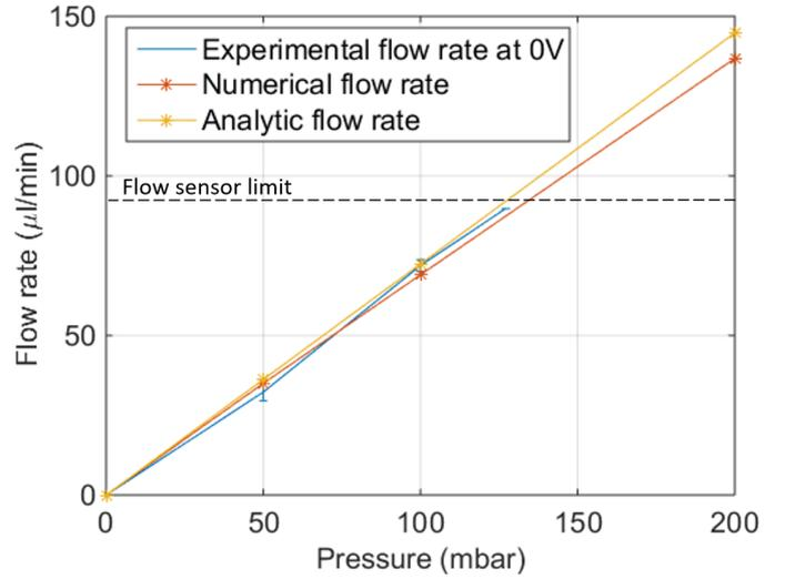
Figure 14: Comparison of the predicted numerical and analytical flow-rates to the measured flow-rates in the microvalve at different pressure levels. The numerical and analytic models assume a valving chamber height of  $11.6 \mu\text{m}$ . Indicated is the flow-sensor limit of  $90 \mu\text{l}/\text{min}$ .
