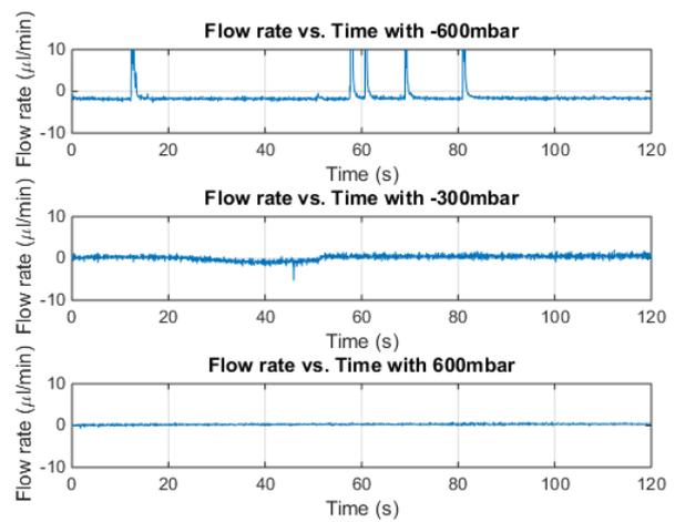
Figure 17: Microvalve stability after being fully closed at different pressure levels.
