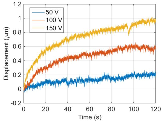
Figure 11: Displacement of the piezo stack over time when the actuation voltage is constant. Different actuation voltages show the corresponding creep rate.
