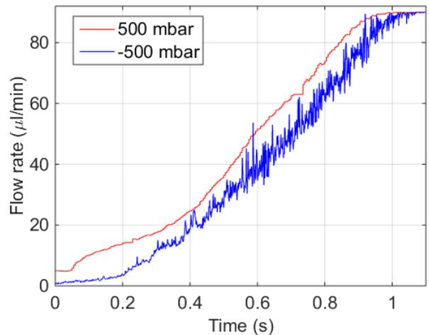
Figure 22: Opening time of the microvalve at 500 and -500 mbar. At 500 mbar vacuum small deviation peaks are observed. The opening times are  $0.79 \pm 0.25$  s (500 mbar) and  $0.86 \pm 0.05$  s (-500 mbar).
