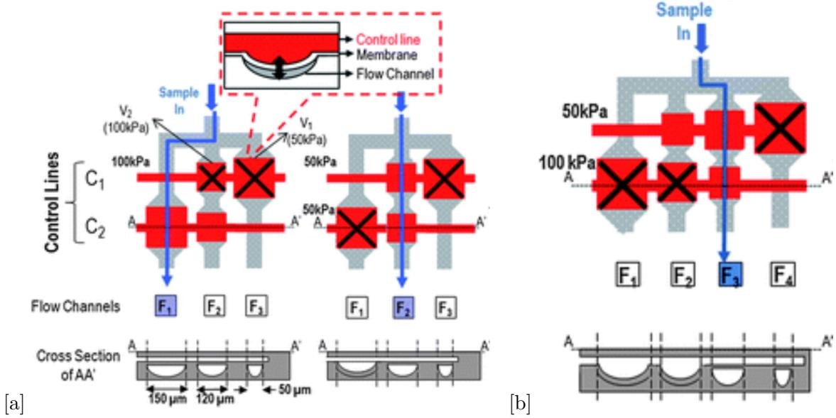
Figure 14: Schematic image of the high radix multiplexers, where the gray lines represent the flow channels and the red lines the control lines. The microvalves are represented as bigger rectangular red block, which when actuated are crossed, the associated actuation pressures are given at the left side of the control lines[24] (a) Ternary multiplexer (b) Quaternary multiplexer.
