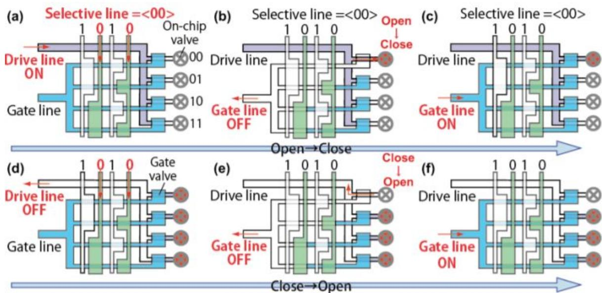
Figure 15: Schematic image of the working principle of the multiplexed control system. The working procedure from opening to closing a On-chip valve is presented in A-C, the working procedure from closing to opening is represented in D-F [25].
