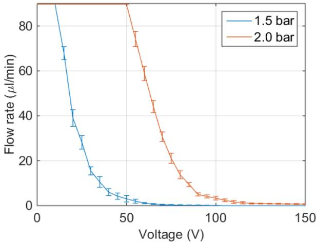
Figure 20: Closing behaviour of the microvalve after using a larger clamping force. Error-bars indicate one standard-deviation of three measurements.
