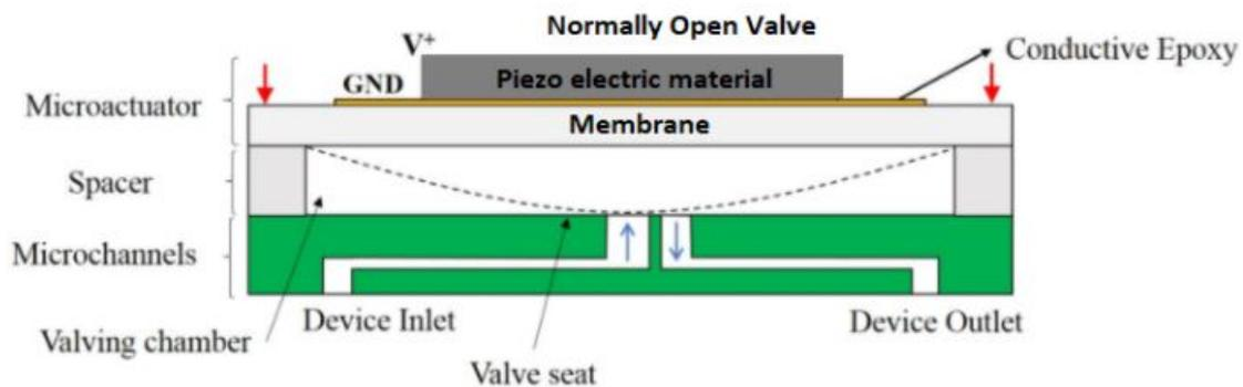
Figure 6: Unimorph NO piezoelectric microvalve [39]
