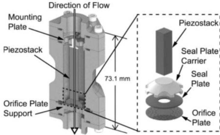
Figure 7: NO piezostack microvalve [41]
