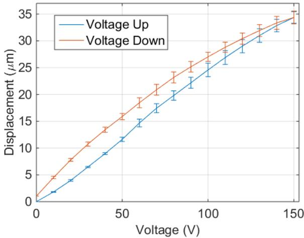
Figure 9: Displacement plot of the piezo stack. The blue curve is measured during voltage-up path and the red curve during voltage-down path. Error-bars indicate one standard deviation of three measurements.
