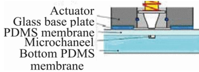
Figure 10: NC electromagnetic microvalve developed by Liu et al. [44]
