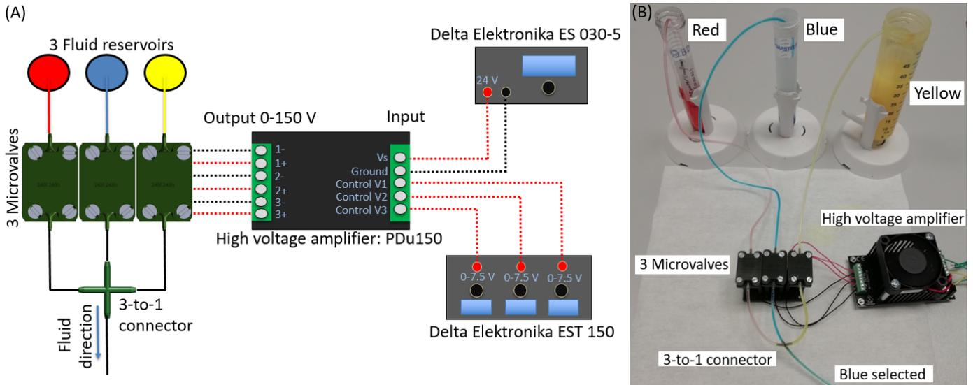
Figure 23: (A) Schematic of the fluid-selector experimental setup (B) Setup of the 3-to-1 fluid selector using three microvalves in parallel. The microvalves are proportionally controlled by the high voltage amplifier. The reservoirs with different colours are connected to the microvalves using a Tygon tubing (ID 1mm). At the output the microvalves are connected with tubings to a 3-to-1 connector. One fluid can be selected forward (blue colored fluid in this Figure).
