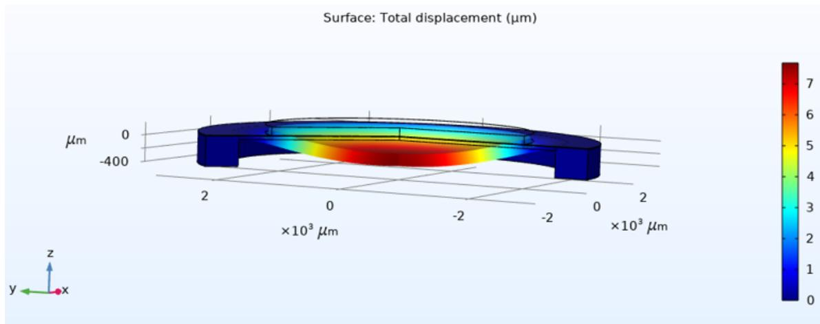
Figure 23: Membrane displacement of a NO- microvalve when 175 V is applied
