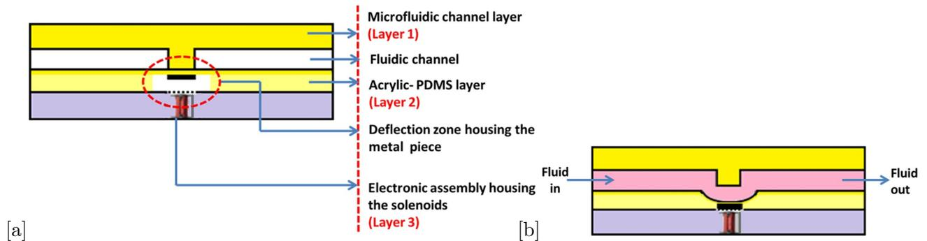
Figure 8: NC electromagnetic microvalve using a metal piece [43] (a) Closed state (b) Open state
