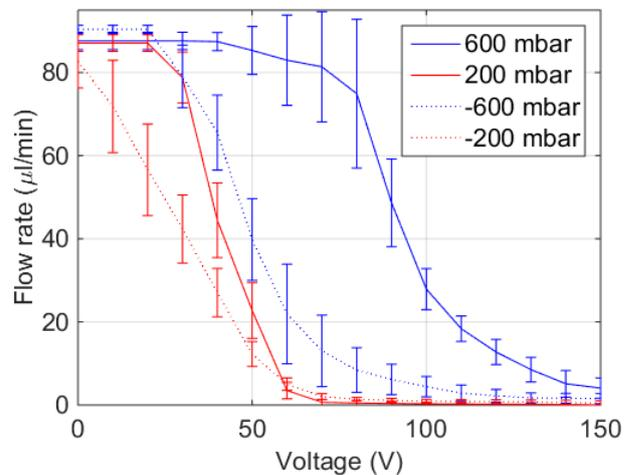
Figure 18: Reproducibility plot for five fabricated microvalves. Each line represents a pressure level and the error bars represent the standard-deviation for five microvalves, with an accuracy of  $<17.89 \mu\text{l}/\text{min}$ . The microvalves are calibrated on  $\pm 70 \mu\text{l}/\text{min}$  at 100 mbar when fully opened.
