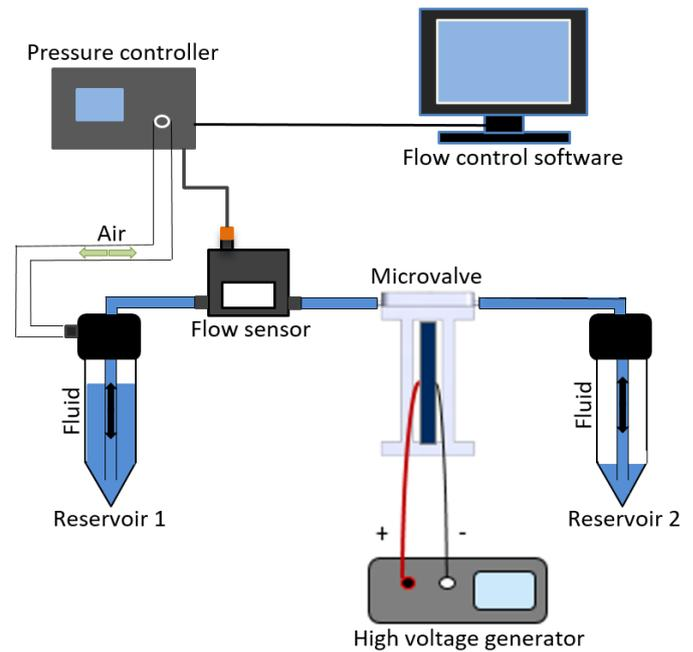
Figure 6: Schematic of the test setup used for measuring the flow-rate. Pressure is applied by the pressure controller to reservoir 1 creating a fluid flow. The flow-sensor measures the flow-rate and the high voltage generator applies voltage to the microvalve. The microvalve can control the fluid flow by adjusting the flow-resistance. The applied pressure and the achieved flow-rates are controlled and visualised in the flow control software.
