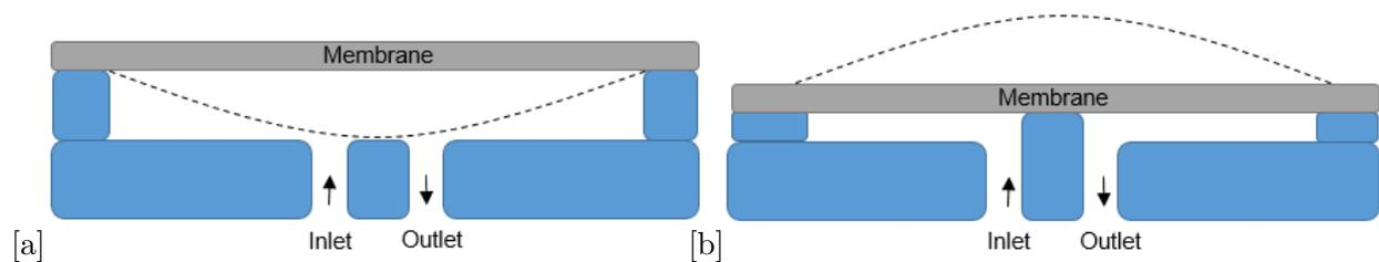
Figure 3: (a) NO microvalve configuration (b) NC microvalve configuration
