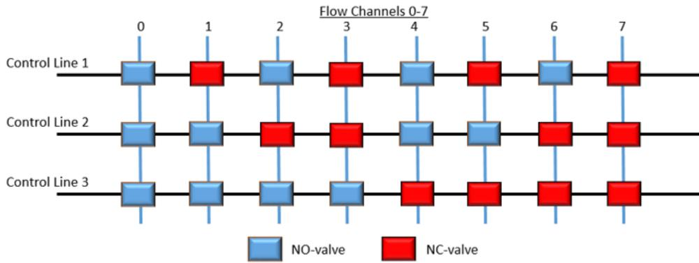
Figure 18: Schematic overview of the binary controlled multiplexer which uses a combination of NO- and NC microvalves. The blue lines represent the flow channels, the black lines represent the control lines.
