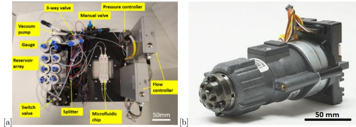
Figure 1: (a) Overview of the microfluidic platform developed by Zhu et al.[14] (b) Switch valve (IDEX MHP7970-500-4)
