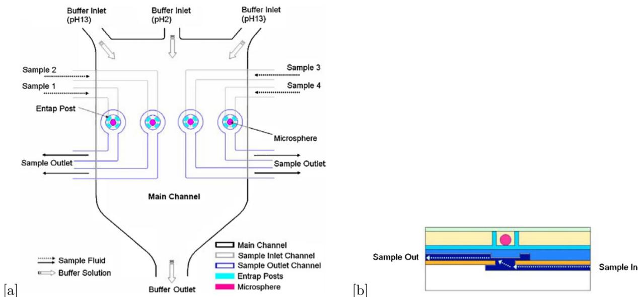
Figure 16: Schematic image of the pH-responsive multiplexer. (a) Gives an overview of the buffer inlets/outlets and the microvalves locations (b) Gives a cross section overview of the microsphere which is pH responsive and can deflect a membrane as a result of the pH responsive swelling [26].
