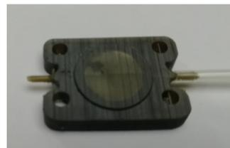
2. Press a tygon tubing with ID of 1 mm over the microfluidic connection
