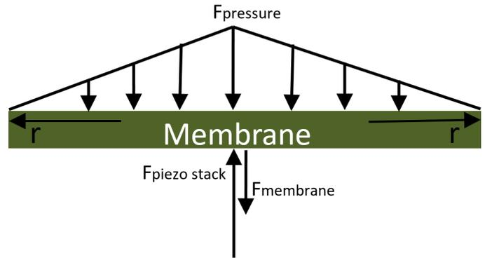
Figure 3: Forces working on the membrane.  $F_{pressure}$  is represented as a triangular distributed load with  $P_1$  as the static pressure at the center (valving chamber inlet) and 0 Pa at the corner. The force as a result of the stiffness of the membrane  $F_{membrane}$  and the force as a result of the piezo stack  $F_{piezostack}$  are represented as a point load.
