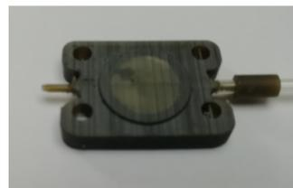
3. Put a ferrule over the tubing to create a leak-tight connection
