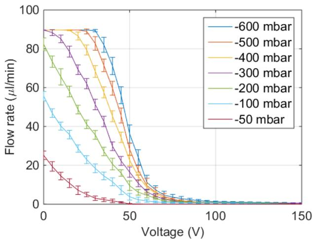
Figure 16: Proportional control of flow-rate at different vacuum levels and actuation voltages. Error-bars indicate one standard-deviation of three measurements, with a precision of  $<4.66 \mu\text{l}/\text{min}$ .
