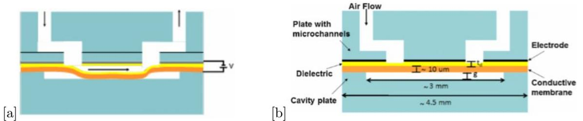
Figure 5: NO electrostatic actuated microvalve [34] (a) Open state (b) Closed state
