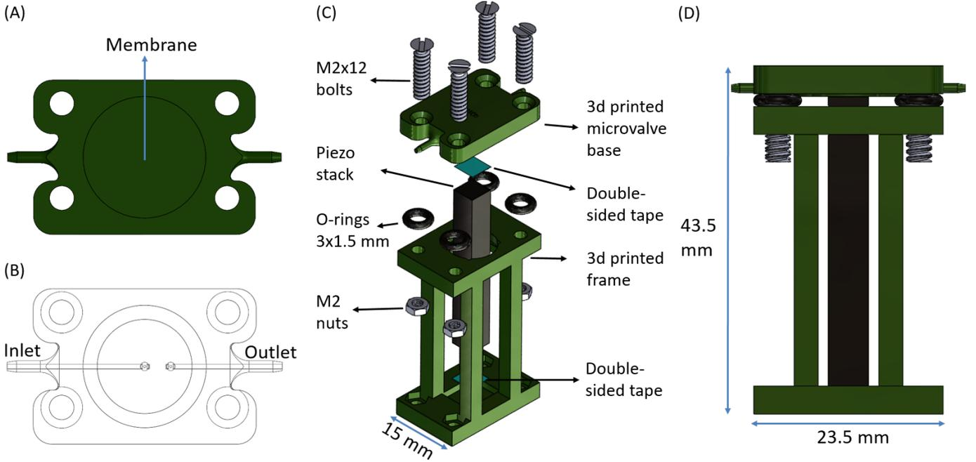
Figure 4: (A) Top view of the microvalve base. The membrane is indicated. (B) Transparent view: internal channels of the microvalve are visible. The inlet and outlet of the microvalve are shown. (C) Exploded view of all the components used during assembling the microvalve. (D) Front view of the assembled microvalve. Also the dimensions are presented.
