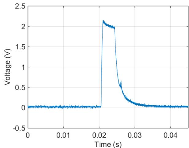
Figure 24: Applied voltage by the portable high voltage amplifier across a resistor connected in series with the piezo stack. Visible are the peak voltage of  $\sim 2.15$  V and the stabilized voltage of 53 mV after charging the piezo stack. The time needed to charge the piezo stack is  $\sim 15$  ms
