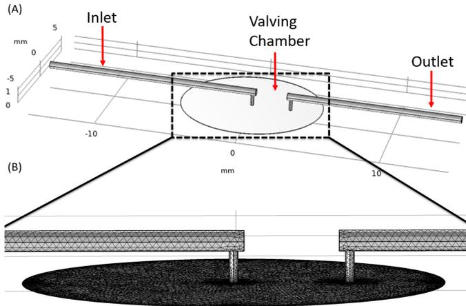
Figure 5: (A) Schematic of the flow path of the microvalve. Indicated are the inlet (where the pressure is applied), the valving chamber and the outlet. (B) Close up of the valving chamber. Also shown is the fine meshing of this feature
