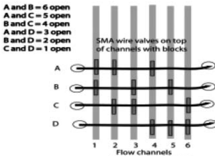
Figure 17: Schematic image of the Shape memory alloy multiplexer. The black lines represent the control lines A-D. the gray lines represent the flow channels. The black blocks on top of the flow channels are the plungers when actuated by the control lines can squeeze/close the flow channels [27].
