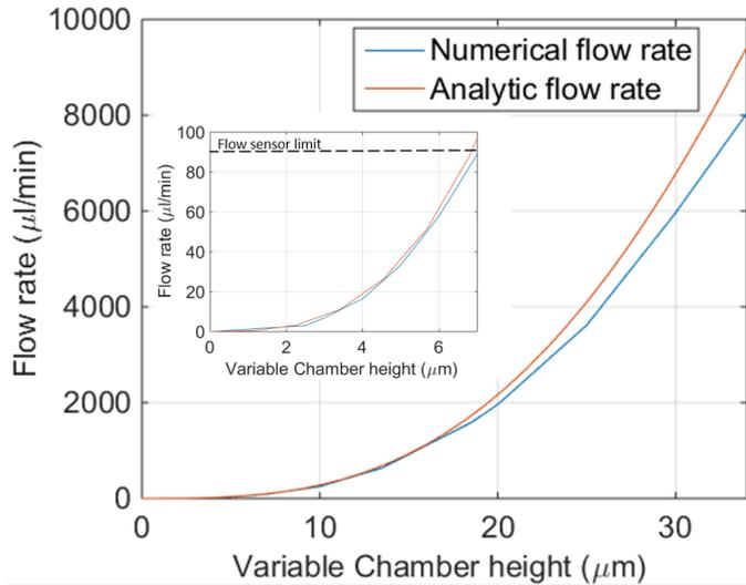
Figure 13: The predicted numerical and analytical flow-rates with varying chamber heights at 600 mbar. The zoom-in plot shows the variable chamber height region with the related flow-rates within the flow-sensor limit of  $90 \mu\text{l}/\text{min}$ .
