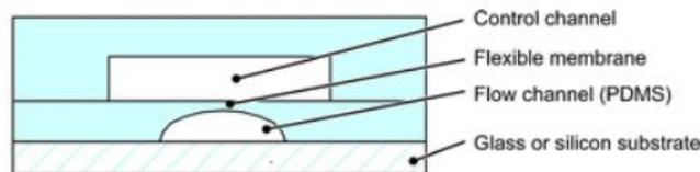
Figure 11: NO pneumatic microvalve [18]
