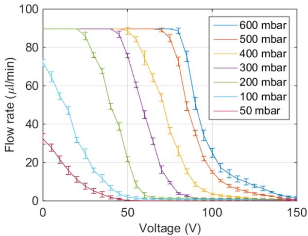
Figure 15: Proportional control of flow-rate at different pressure levels and actuation voltages. Error-bars indicate one standard-deviation of three measurements, with a precision of  $<3.63 \mu\text{l}/\text{min}$ . Clearly visible is the flow-sensor limit of  $90 \mu\text{l}/\text{min}$ .
