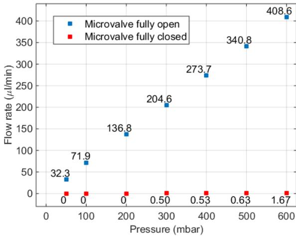
Figure 19: Flow-rate of the microvalve in the fully open and in the fully closed position at different pressure levels. The numbers indicate the flow-rates at the data points. Leakage-rates: 0% (50 mbar), 0% (100 mbar), 0% (200 mbar), 0.24% (300 mbar), 0.19% (400 mbar), 0.18% (500 mbar), 0.41% (600 mbar).
