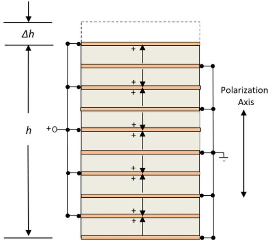
Figure 2: Schematic of the piezo stack. The grey layers represent the piezoelectric material and the orange layers represent the metal layers. The black arrows indicate the poling direction. The dashed lines show the expansion  $\Delta h$  of the piezo stack with original length  $h$ .
