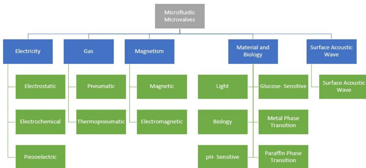
Figure 2: Active microfluidic microvalves actuation mechanisms divided in 5 groups based on their main actuation characteristic [28]
