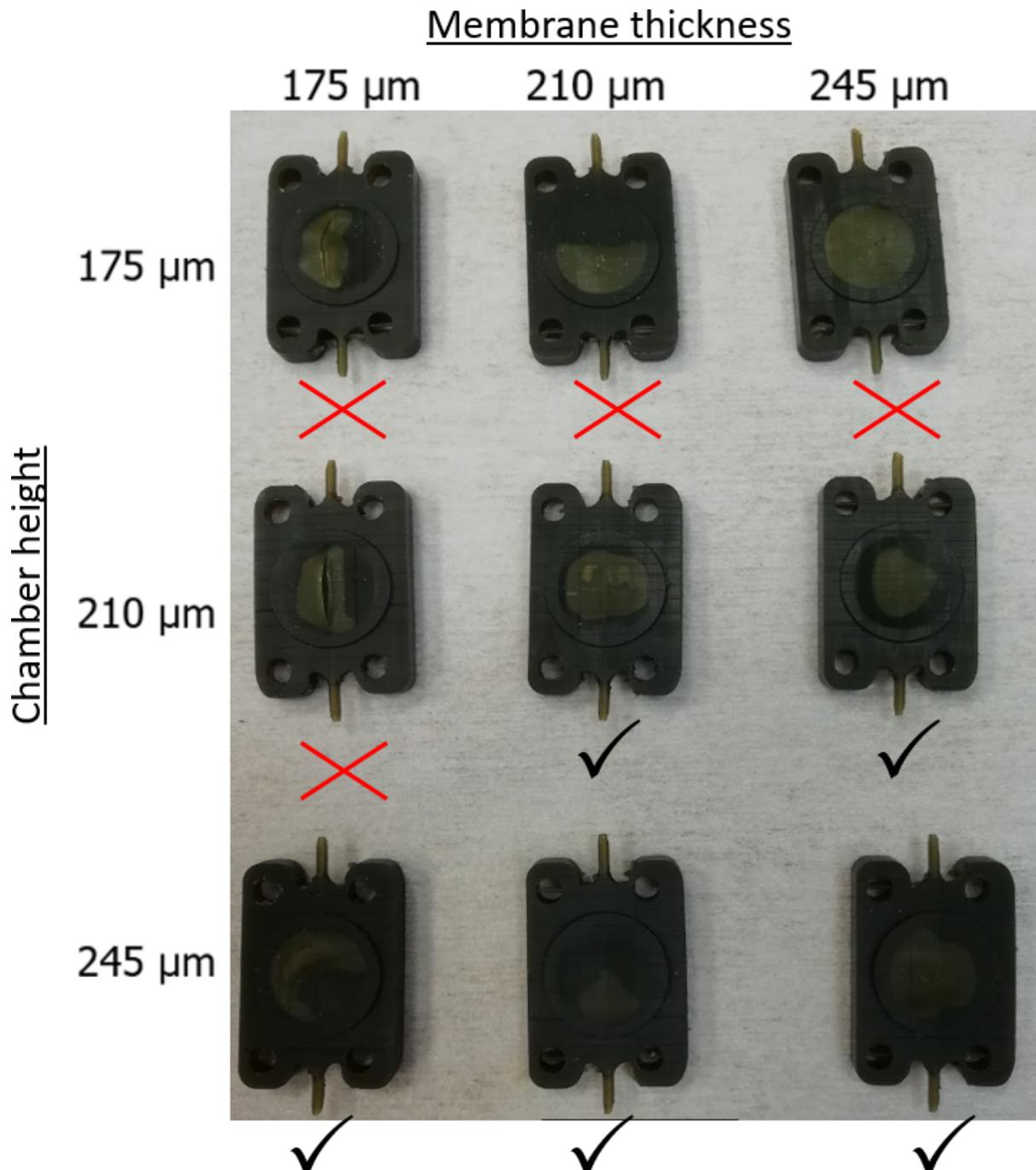
As can be seen in the figure above the damaged/not intact membranes are marked with a red cross, while the intact membranes are marked with a check mark. An intact membrane is printed when at least a chamber height of 210  $\mu\text{m}$  and a membrane thickness of 210  $\mu\text{m}$  is used. During testing a chamber height of 245  $\mu\text{m}$  and a membrane thickness of 245  $\mu\text{m}$  is used to guarantee a robust membrane.
