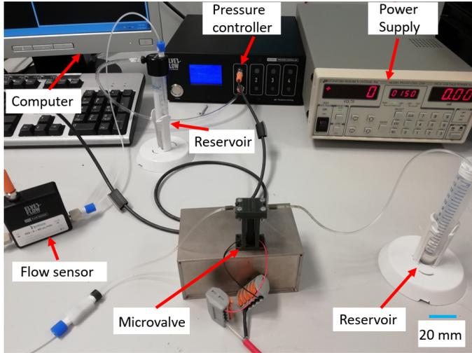
Figure 12: Microvalve test-setup. The microvalve is placed in the centre on a stage to compensate for the height differences with the fluid levels in the reservoirs.
