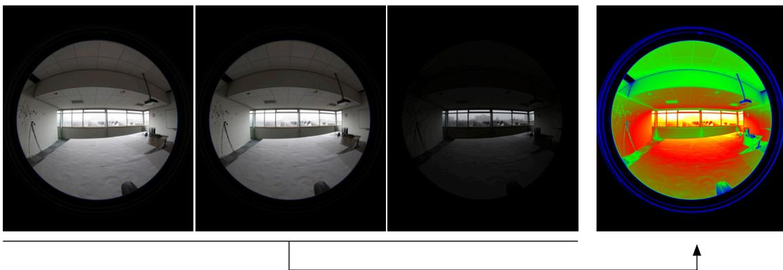
**Figure 2.4** An under-, normal- and overexposed fish eye image, resulting in a luminance false-color map.
