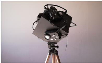
**Figure C.1** The top row presents the iterative process of the making off the cubic illuminance meter. The final design of the cubic illuminance meter fixated on a tripod is presented in the line below. The flat top side of the cube makes it possible to orient the cube using a spirit level.
