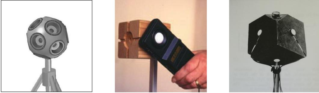
**Figure 3.5** Tools to measure the light field: (left) The custom-made plenopter of Mury with 12 photodiodes (Mury, 2009) (middle) A Cubic Illuminance meter using a single Lux Meter (Cuttle, 2009). (right) The cubic illuminance meter of Xia *et al.* (2016-III) with six photodiodes (right).
