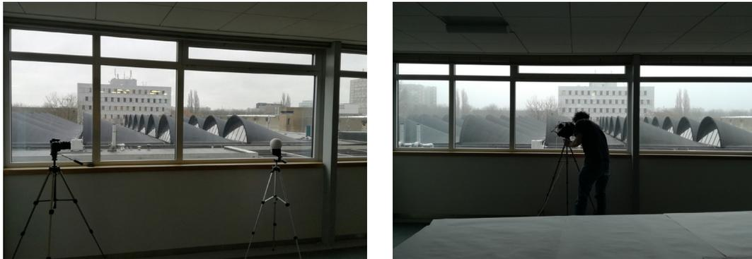
**Figure 8.3** (left) An impression of a luminance camera on a tripod photographing a hockey ball on a tripod, and (right) the installation of the cubic illuminance meter on a tripod at grid point A1. The left image shows the in white paper folded table as well.
