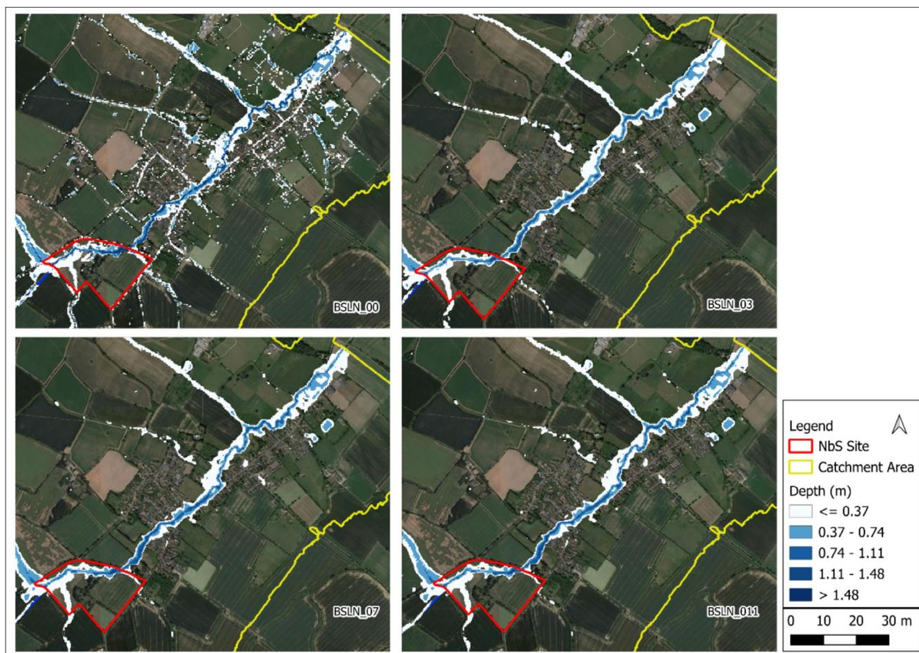
**FIGURE 4** | Flood depth within Risely under the simulated SGS frequencies.
