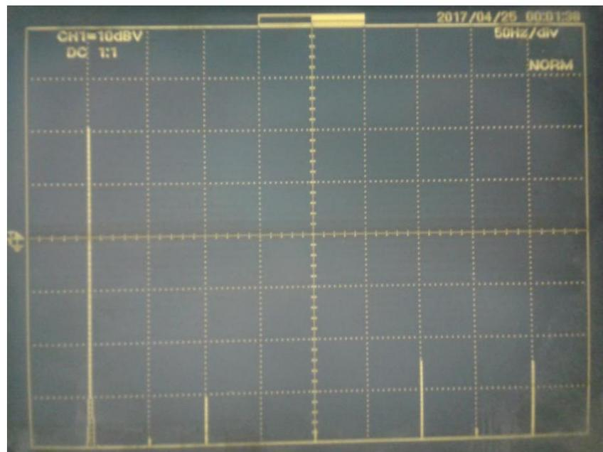
Figure 31. Harmonic spectra with 3<sup>rd</sup> harmonic amplitude strongly reduced and 7<sup>th</sup> harmonic slightly reduced. Levels considered to be under the IEC standard maximum levels.
