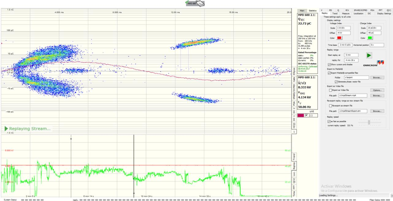
Figure 43. Screen shot of the OMICRON software where the data exported to the Matlab function is the selected part between the cursors in the lower graph and the PD pattern generated during this time is shown in the upper graph. On the right-hand side of the figure, the mean real time PD event charge value and the applied voltage level can be seen, as well as the control screen for the replay of the recording done during the experiment.
