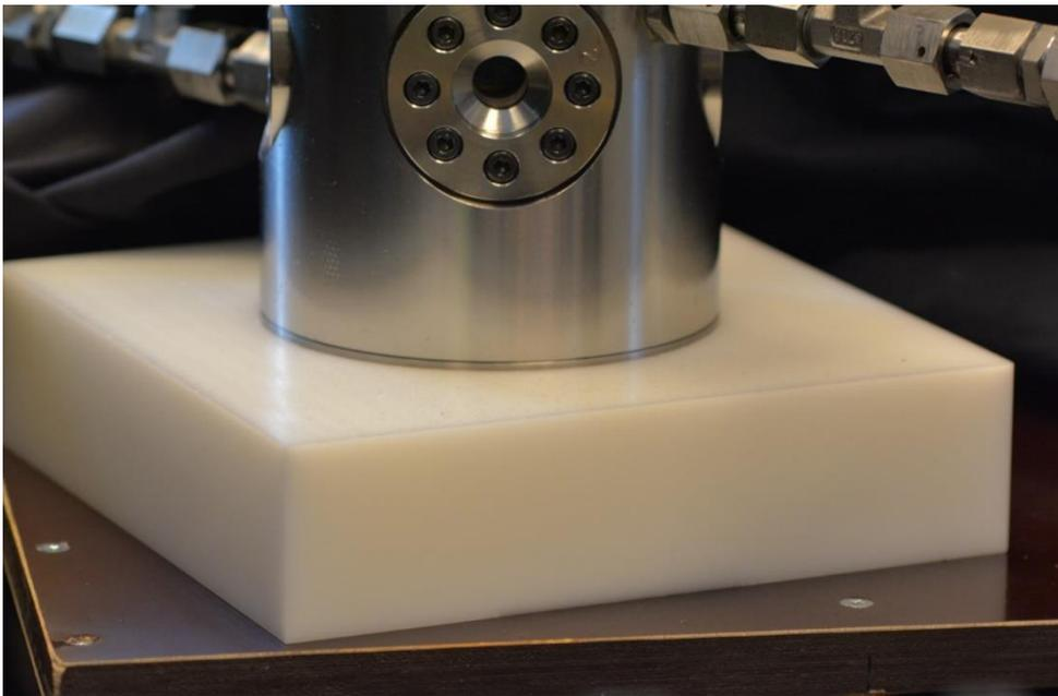
*Figure 25. Insulating and stabilizing designed base for the pressure vessel.*
