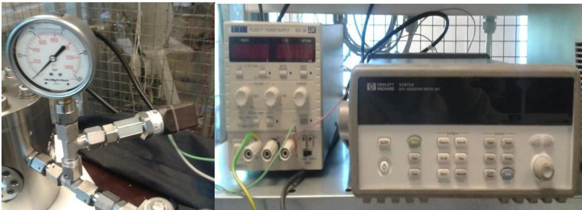
Figure 32. Barometer and pressure sensor (left). Pressure sensor power supply and data logger (right)
