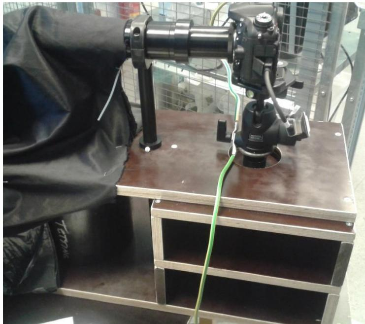
*Figure 27. Insulating and stabilizing designed base for the NIKON camera and the long-distance microscope lens*
