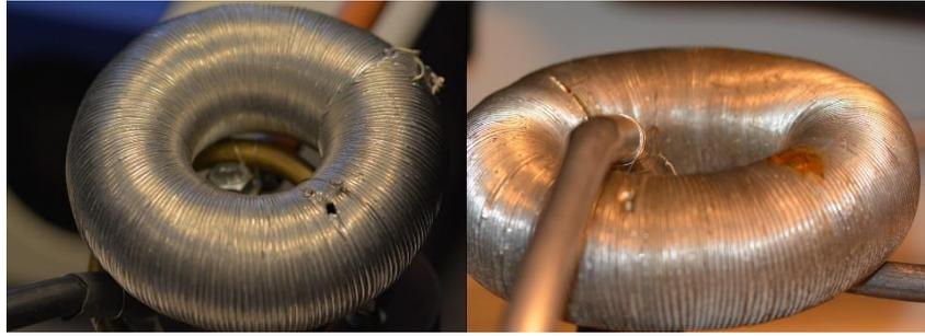
*Figure 26. Toroids installed in the transformer connection point (left) and pressure vessel HV electrode connection point (right)*
