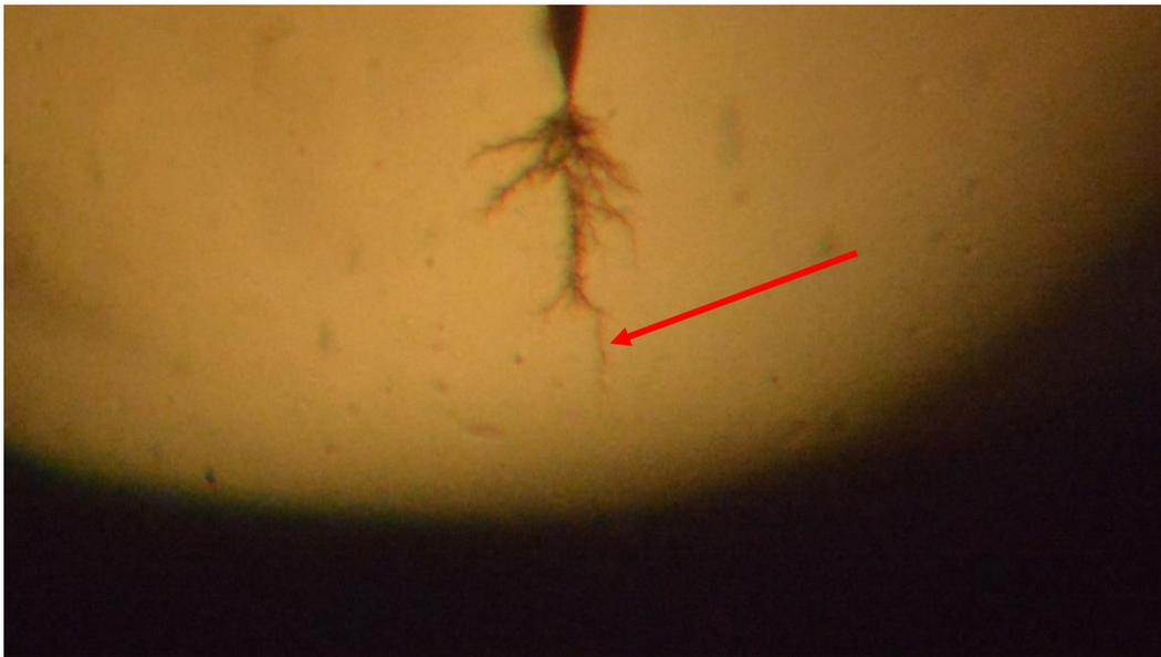
*Figure 14. Picture taken during one of the initial tests of this thesis experimental part. “Leader” branch formed previous to breakdown occurrence.*
