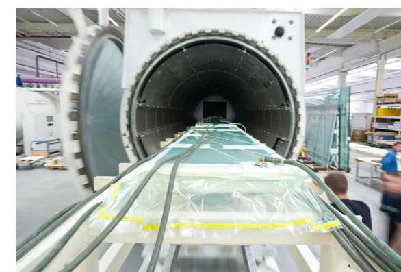
Lamination of the components into one element / panel
