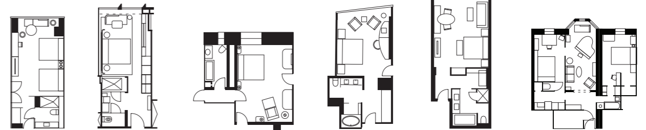
Marriott Marquis 4.2 x 9.2 m 40 m 2 Equinox Hotel 4.2 x 10 m 42 m 2 The Plaza 7.2 x 6.4 m 43 m 2 Aria Rooms & Suits Las Vegas* 5.2 x 9.6 m 48 m 2 Four Seasons Orlando* 4.5 x 12.5 m 55 m 2 Chelsea Hotel 8.4 x 7.8 m 74 m 2
