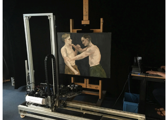
Figure 12. The scanner used for scanning the painting
