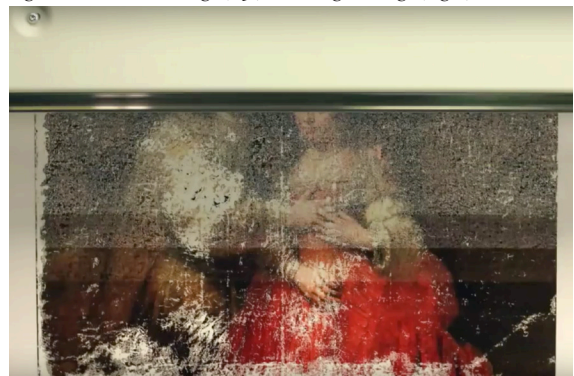
Figure 14. The Océ printer builds the painting up in layers
