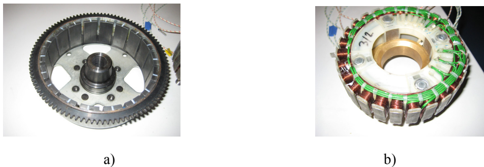
Figure 2.1. A PM machine for vessel application: a) rotor, b) stator.
