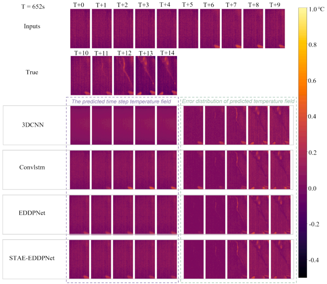
Fig. 15. The prediction results and error distribution plots of each model for the test instance corresponding to loading time point c of sample A39.
