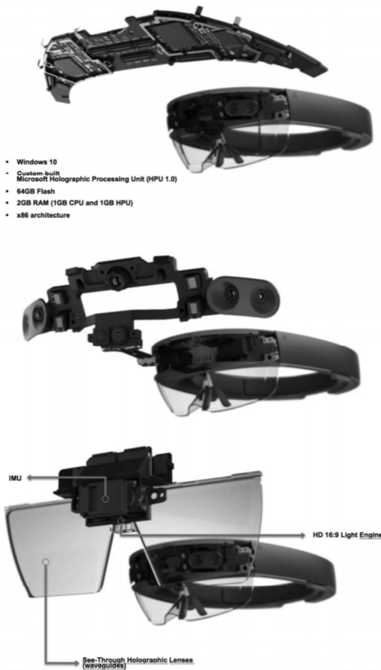
Figure 2.14: Microsoft HoloLens' Architecture [Kress and Cummings, 2017]
