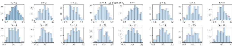
Figure 5.7: Distribution of biases for up movements ( $r_t \geq 1$ ) for  $p_a$  for all feature channels ( $S = 16$ ) of OBNet in the predictive setting. Plots with a higher opacity are the ones that the network weighs more.
