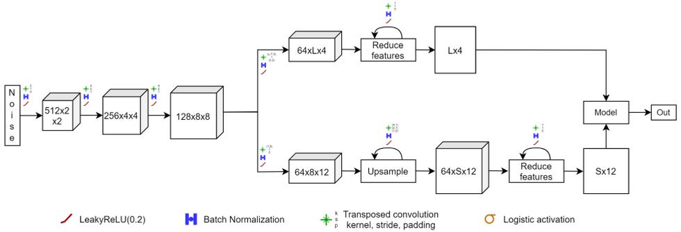
Figure 3.3: A schematic of the generator. The 3D blocks represent the matrices at various stages throughout the network, noted using  $C \times W \times H$ . The upper branch of the network represents the learned initial values and the lower branch of the network represents the learned weights for combining rates and transition probabilities.
