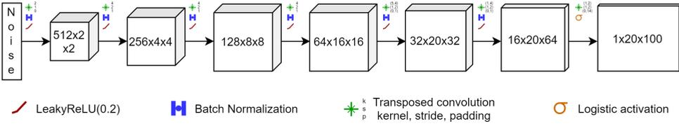
Figure 4.3: The architecture of the generators of DCGAN and WGAN in the generative setting. The 3D blocks represent the images at various stages throughout the network, noted using  $C \times W \times H$ . The flat rectangles represent vectors of dimension  $C$ .
