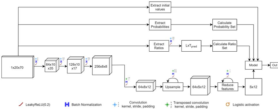
Figure 3.6: A schematic of the generator in the predictive setting. The 3D blocks represent the images at various stages throughout the network, noted using  $C \times W \times H$ .
