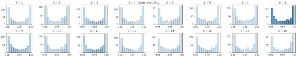
Figure 5.5: Distribution of down rates ( $r_t \leq 1$ ) for  $p_a$  for all feature channels ( $S = 16$ ). Plots with a higher opacity are the ones that the network weighs more.
