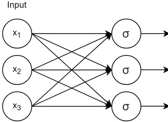
Figure 2.1: An example of an single layer perceptron with three hidden neurons and an input of dimension 3. Each neuron receives the input vector as its input. The outputs of the neurons can be fed into the next layer of neurons, in which case each neuron in the next layer would similarly receive the output vector of this layer.
