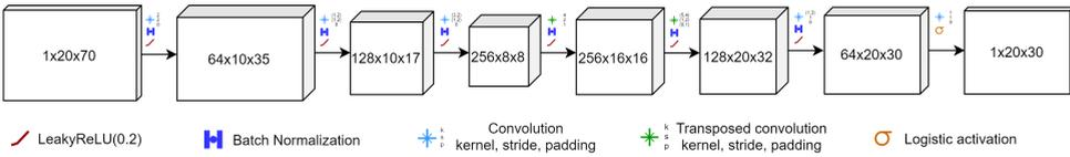
Figure 4.4: The architecture of the generators of DCGAN and WGAN in the predictive setting. The 3D blocks represent the images at various stages throughout the network, noted using  $C \times W \times H$ . The flat rectangles represent vectors of dimension  $C$ .
