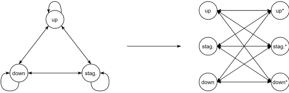
Figure 3.4: Translating a fully connected graph with three states to a fully connected bipartite graph with six states.
