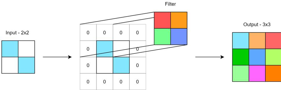
Figure 2.2: A transposed convolution operation on an input matrix of  $2 \times 2$ . It gets padded with zeroes and a  $2 \times 2$  filter is applied with stride 1. The resulting output is a  $3 \times 3$  matrix.
