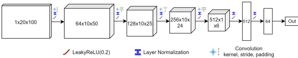
Figure 3.7: A schematic of the critic. The 3D blocks represent the images at various stages throughout the network, noted using  $C \times W \times H$ . The flat rectangles represent vectors of dimension  $C$ .
