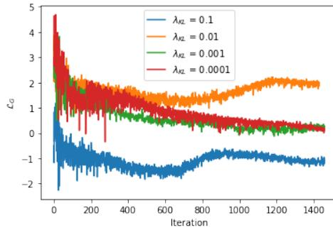
Figure 5.14: The loss of the generator  $\mathcal{L}_G$  over the training iterations for various values of  $\lambda_{KL}$
