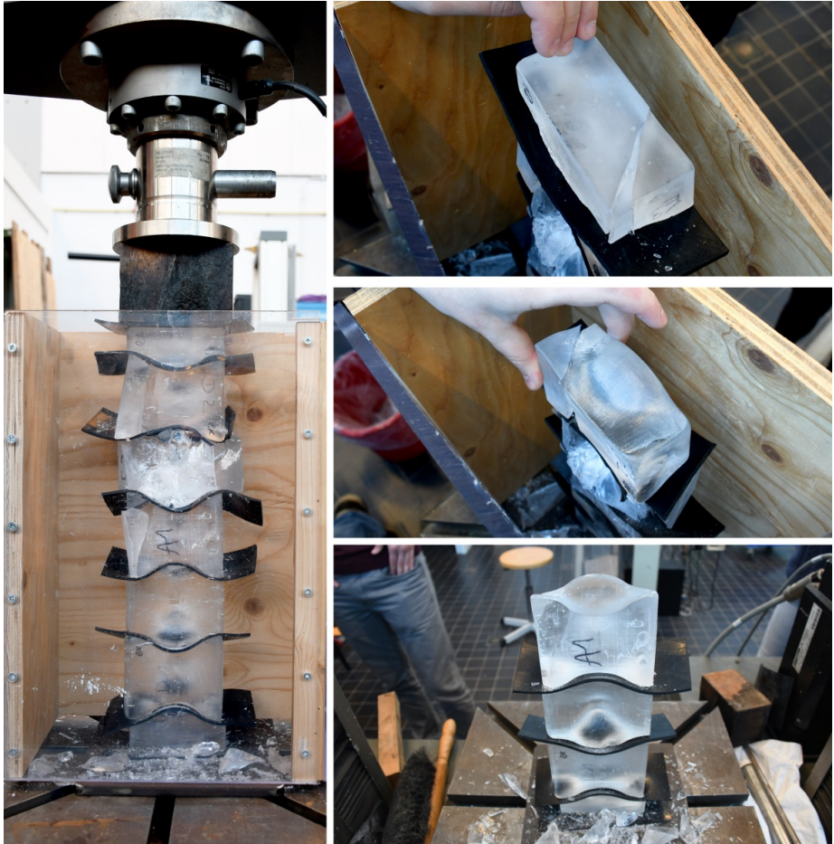
Figure 26: Specimen B after failure. Left: overview; Right: crack patterns in blocks a, b and d (top down). Block c was completely fragmented and could not be retrieved after the testing.
