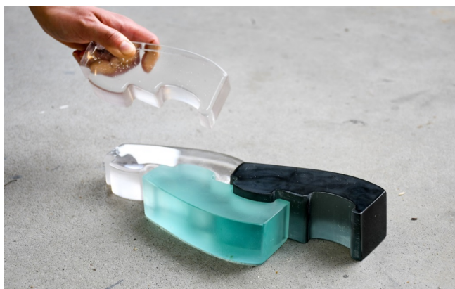
Figure 8: Type D prototype made of clear glass, recycled float glass (teal) and recycled Cathode Ray Tube (CRT) screen (black)
