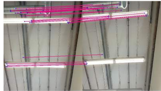
(b) Feature matching with SIFT detector and SURF descriptor
