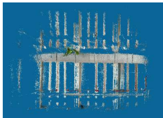
(b) Point cloud of room 08.02.00.560, reconstructed from overlapping images
