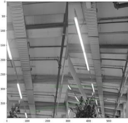
(b) Feature detection with SIFT and feature matching with FLANN
