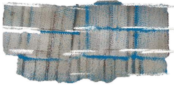
Figure 5.5.: Point cloud of room 08.02.00.430, where the user stumbled during the acquisition
