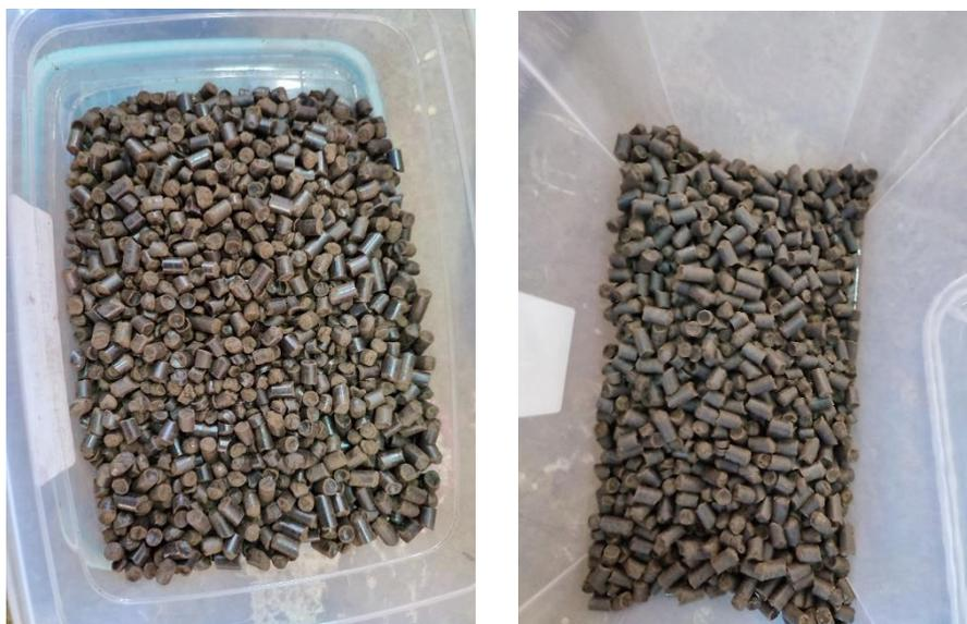
**Figure 19.** Pictures of torrefied hay pellets. On the left, there are the ones with 5% PE and on the right with 10% PE.
