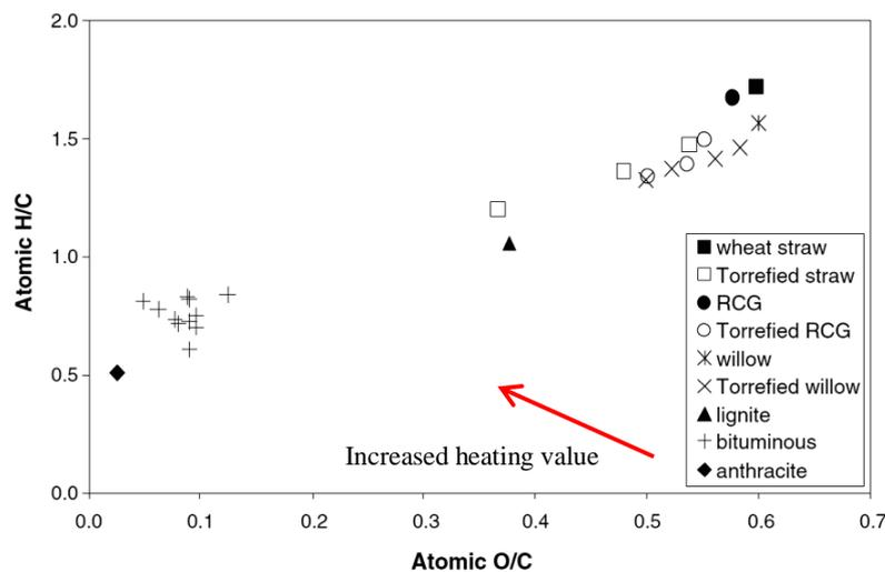
Figure 3. Comparison of coal's atomic H/C and O/C ratio with raw and torrefied biomass. (Bridgeman et al., 2008)
