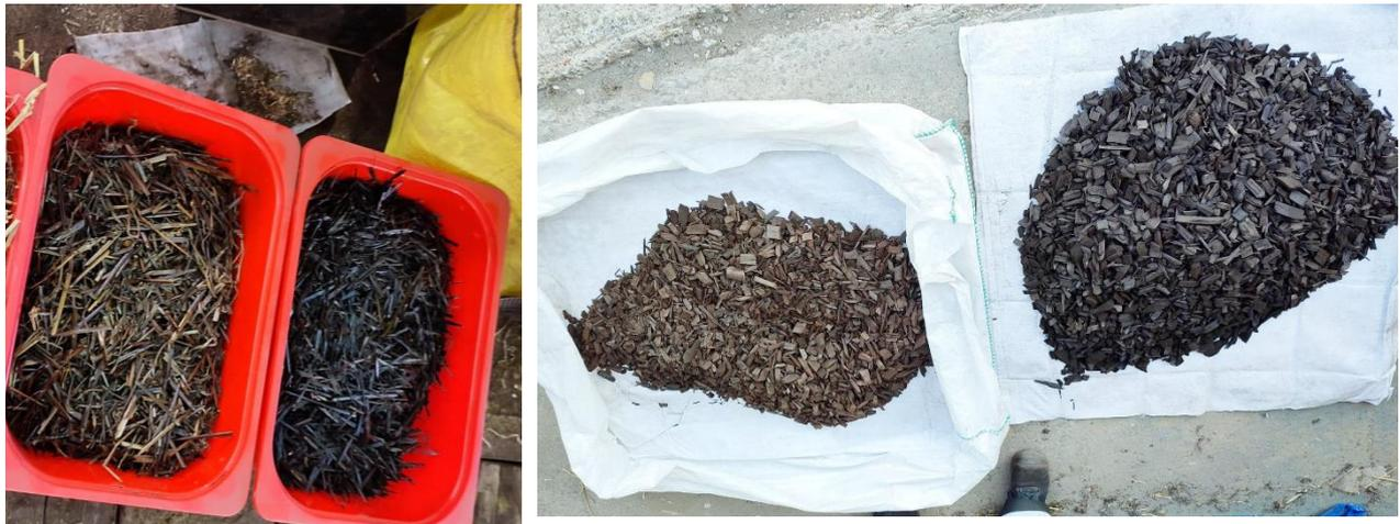
**Figure 8.** Straw (left) and woodchips (right) torrefaction products after the 240 °C and 270 °C runs.
