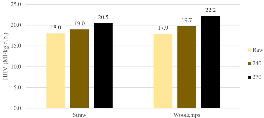
**Figure 12.** Effect of torrefaction on HHV on dry basis to wheat straw and woodchips.
