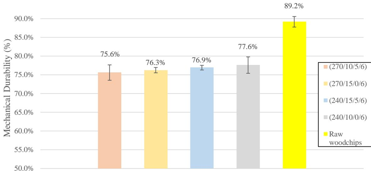
**Figure 15.** Mechanical durability of torrefied and raw woodchip pellets.
