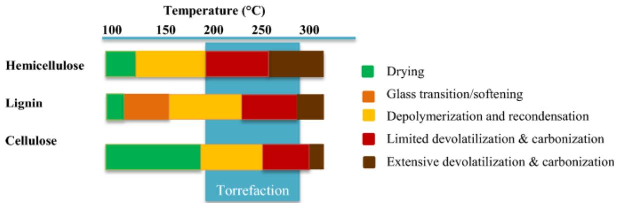
Figure 2. Basic stages of torrefaction and their effect on hemicellulose, cellulose and lignin (Negi et al., 2020).
