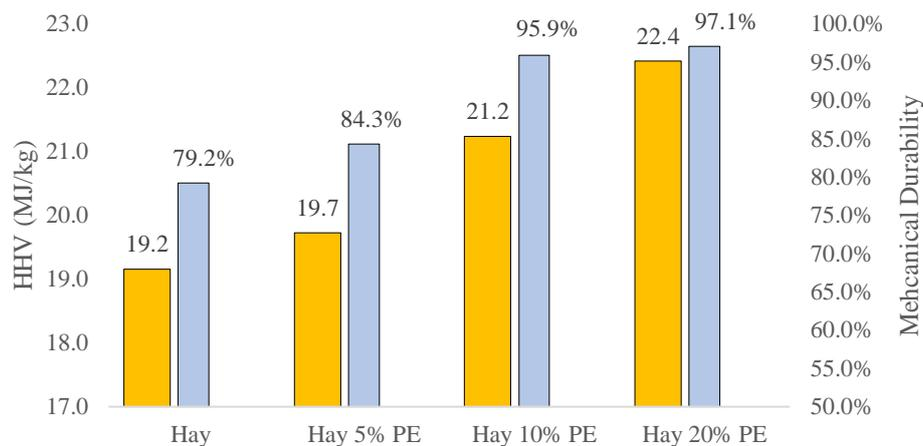
**Figure 18.** Plastic concentration effect on torrefied hay pellets' mechanical durability and HHV on dry basis.
