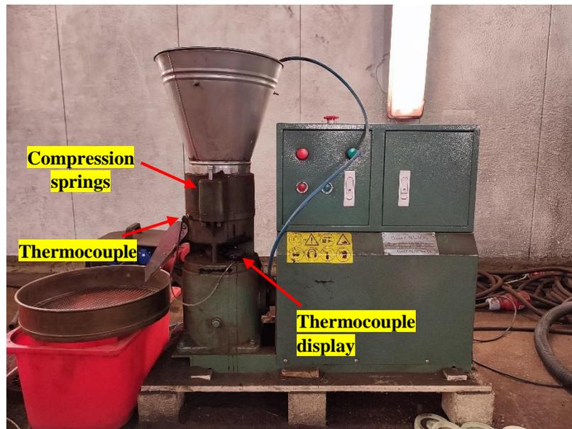
**Figure 7.** Pelletizing setup (the attached thermocouple is seen with the display of temperature).
