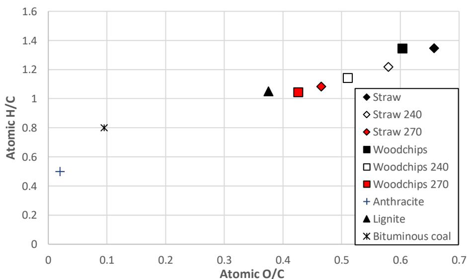
**Figure 11.** Van Krevelen diagram for the torrefied biomass samples and comparison with commodity fuels.
