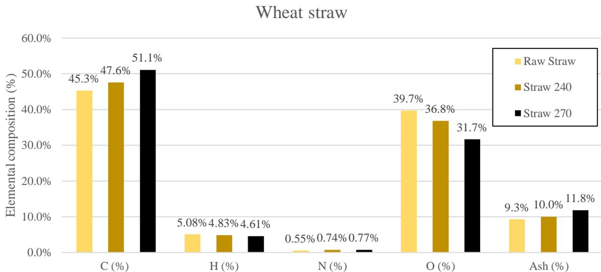
**Figure 9.** Percentage difference in elemental composition for wheat straw after torrefaction.
