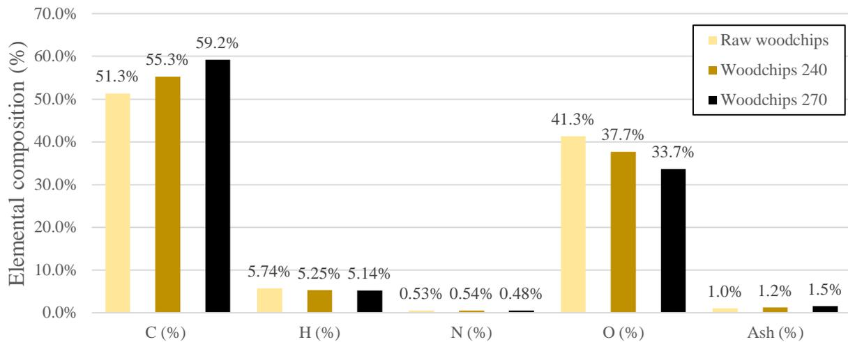
**Figure 10.** Percentage difference in elemental composition for woodchips after torrefaction.
