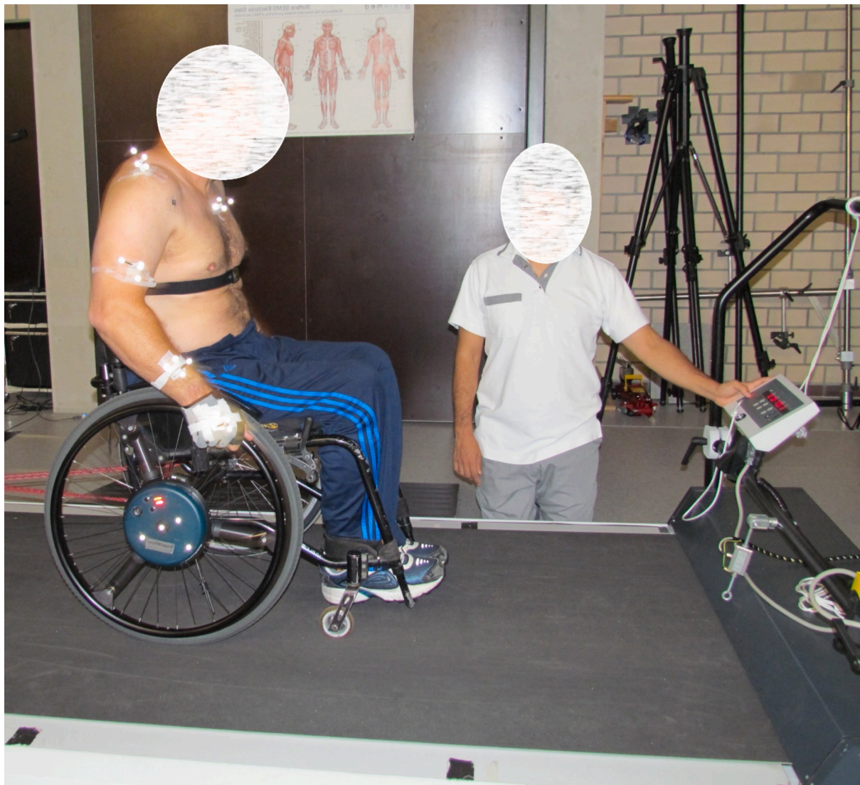
Fig. 2. The setup for the registration of UE-kinematics and WCP-kinetics, before and after the overground fatiguing protocol. A pulley system was used to add extra weight to arrive at 25 W or 45 W power output for all participants. For each participant, the required weights were determined from a drag test measuring rolling resistance force.
