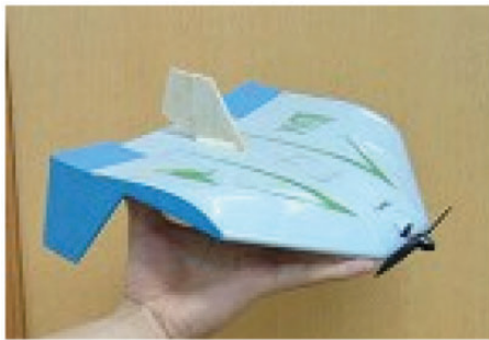
Figure 9. Fixed-Wing MAV with a trapezoidal wing platform.
