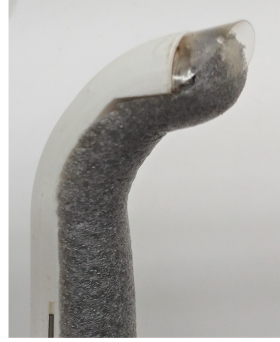
FIG. 10: One of the fingers of the 4FH, including the nail (transparent) at the finger tip and the compliant material (grey) on the inside of the finger
