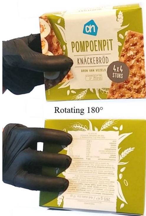
FIG. 17: Performing one of the tasks of the modified AHAP. The object must be rotated 180^\circ and back for three times. Score is based on whether the object is dropped or shows motion with respect to the gripper.
